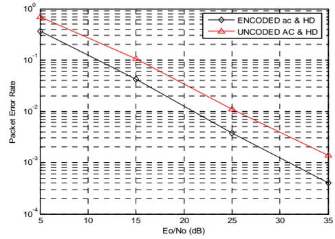
Fig.(8): PER vs. SNR over fading channel (AC&HD with and without FEC)
