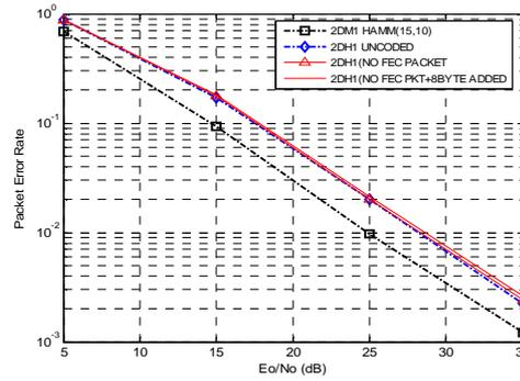
Fig.(9): PER vs. SNR over fading channel (EDR& Proposed cases)
