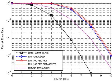
Fig.(6): PER vs. SNR over AWGN channel (EDR and proposed cases)
