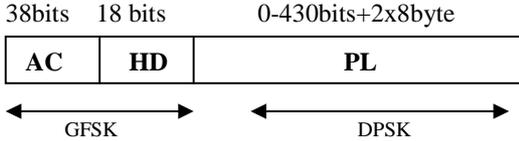
Fig. (4): Adaptive Bluetooth EDR packets format (2DH<sub>1</sub>)
