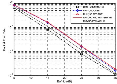
Fig.(10): PER vs. SNR over fading channel (classic and proposed case)
