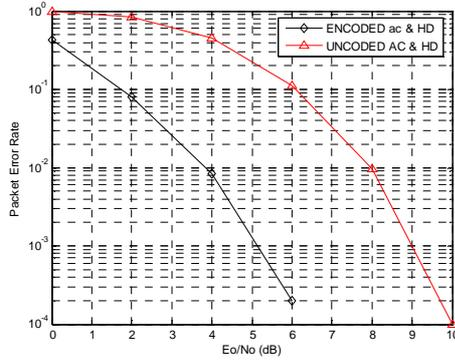
Fig.(5): PER vs. SNR over AWGN channel (AC&HD with and without FEC)
