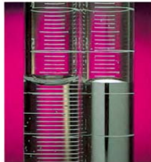
Figure 13-9 The meniscus, as observed in glass tubes with water and with mercury.
