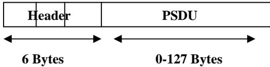
Figure 1: ZigBee packet format
