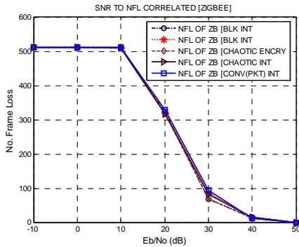
Figure 8: NFL vs. SNR over correlated fading channel
