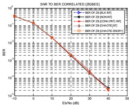
Figure 9: BER vs. SNR over correlated fading channel
