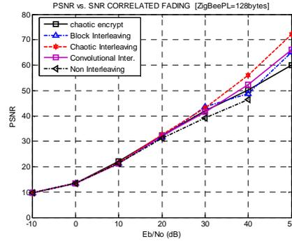
**Figure 5:** PSNR vs. SNR for ZigBee network
