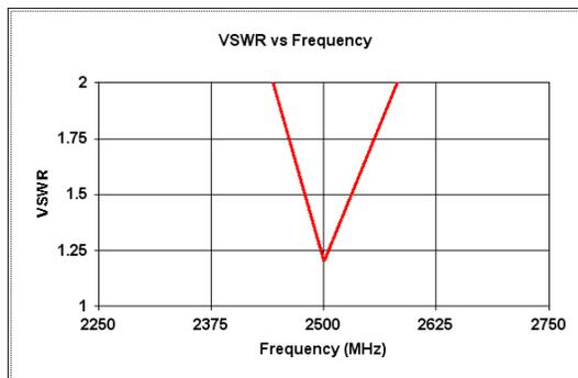
Figure 7 Variation of VSWR versus frequency for conventional inverted F wire antenna
