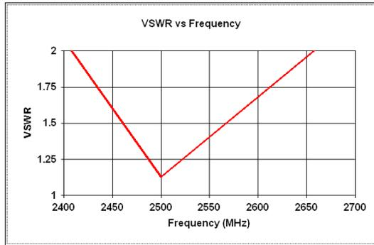
Figure 11 Variation of VSWR versus frequency for modified inverted F wire antenna (MIFA2)
