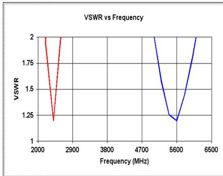
Figure 2 Variation of VSWR versus frequency for rectangular meander wearable antenna
