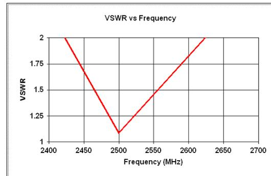
Figure 9 Variation of VSWR versus frequency for modified inverted F wire antenna (MIFA1)
