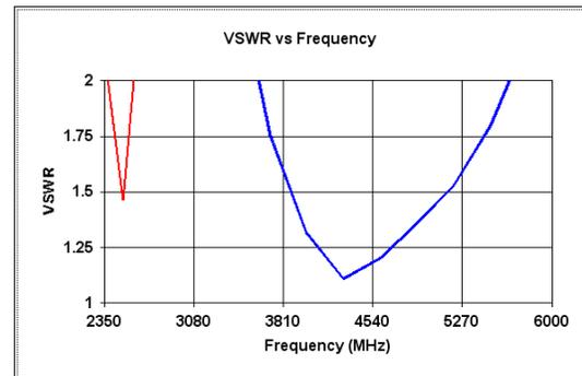
Figure 14 Variation of VSWR versus frequency for the proposed configuration of two inverted F wire antenna (2-IFA))
