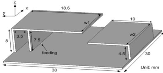
Figure 5 Geometry of the antenna that proposed by C. H. See [9].
