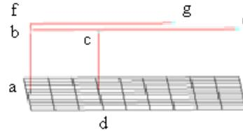
Figure 8 Modified inverted F wire antenna (MIFA1)
