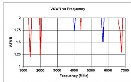
Figure 4 Variation of VSWR versus frequency for triangular meander wearable antenna
