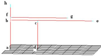
Figure 10 Modified inverted F wire antenna (MIFA2)
