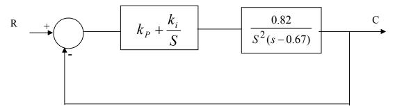
3. Consider the system shown in figure. Design a controller that gives the system zero steady state error for a velocity input and dominant closed loop poles with damping ratio of 0.707. Estimate a unit step response of the compensated system.
