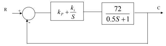
2. Design a PI controller to the shown system which has desired poles of  $(S = -0.56 \pm j0.4)$ .
