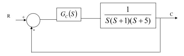
**8.** For the system shown in figure design a PID controller using a Ziegler-Nichols method for tuning the coefficients and compute the resulting step response of the closed loop system.
