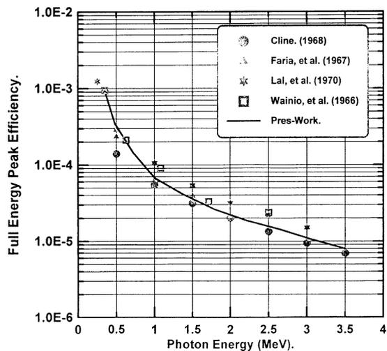
Fig. 8. Comparison of present calculations for full-energy peak efficiency with experimental values measured by Cline (1968) and theoretical results of Lal and Iyengar (1970), Wainio and Knoll (1966) and Faria and Levesque (1967) using the Monte Carlo method. The experiment and simulations concerned a 2 cm<sup>3</sup> Ge (Li) detector with axial point source at a height of 5 cm above the front face of the detector.
