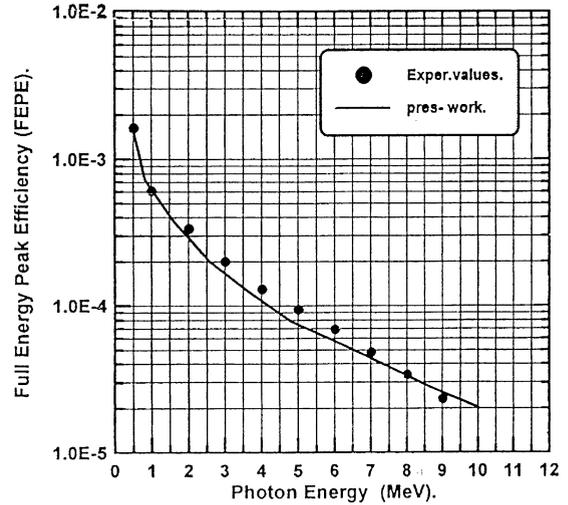
Fig. 4. Comparison of present calculations for full-energy peak efficiency with experimental values measured by Young et al. (1971) for a 50 cm<sup>3</sup> coaxial Ge (Li) detector and an axial point source at a height of 10 cm above the front surface of the detector.
