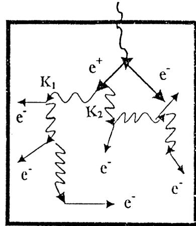
Fig. 2. Schematic behavior of annihilation photons in the detector.
