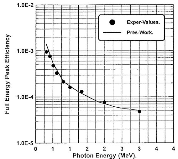
Fig. 5. Comparison of present calculations of full-energy peak efficiency with experimental values measured by Schotzig et al. (1973) for a 44 cm<sup>3</sup> Ge (Li) detector and an axial point source at a height of 16 cm above the front surface of the detector.
