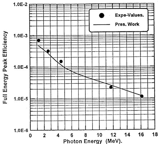
Fig. 3. Comparison of present calculations for full-energy peak efficiency with experimental values measured by Cecil et al. (1985) for a 65 cm<sup>3</sup> Ge (Li) detector and an axial point source at a height of 13 cm above the front surface of the detector.
