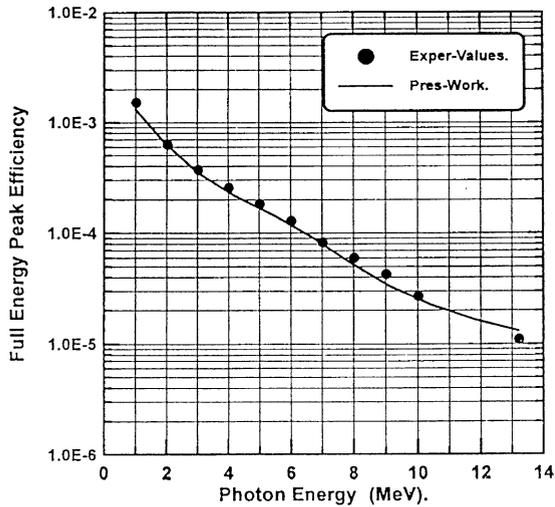
Fig. 7. Comparison of present calculations for full-energy peak efficiency with experimental values measured by Waibel and Grosswendt (1976) for a 26 cm<sup>3</sup> true coaxial Ge (Li) detector, with an axial point source at a height of 4.83 cm above front face of detector.
