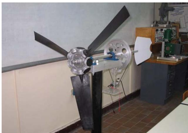
Fig.(14) Experimental setup of wind energy system.
