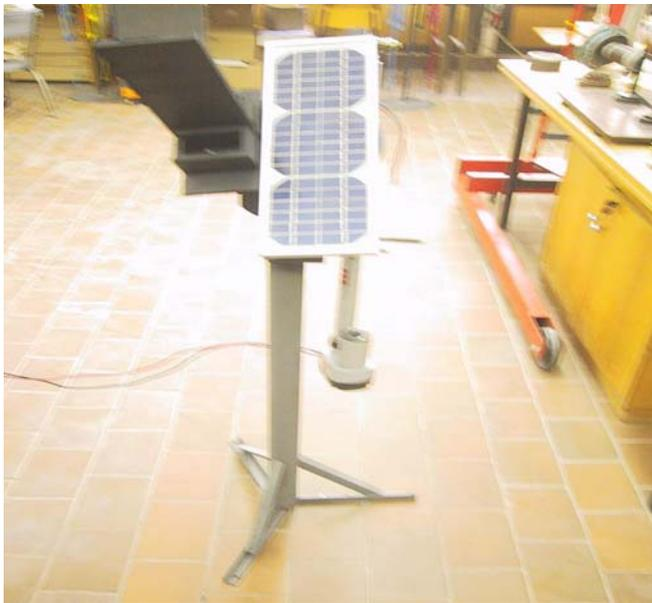
Fig.(9) Mechanical setup of the sun tracking system.
