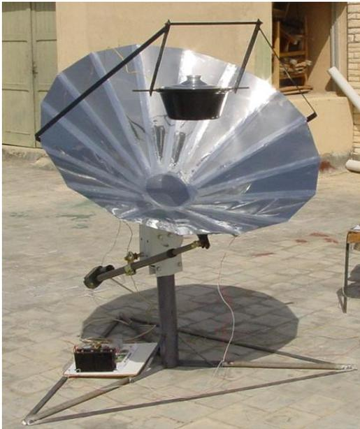
Fig. 1 The solar cooker with sun tracking system
