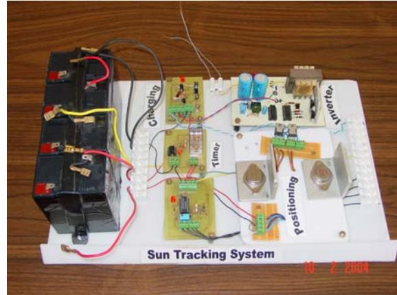
Fig. 2. Sun tracking control circuit.
