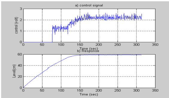
Fig. 26 Level response with adjusted output scale
