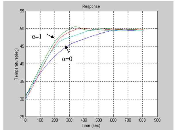
Fig. 15 Different responses for different values of  $\alpha$  at gain = 1
