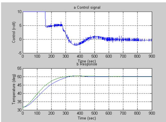
Fig. 24 Actual response using model reference supervisor controller at flow 80%
