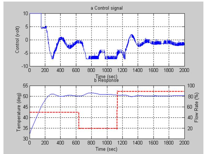
Fig. 20 Actual response using supervisor controller when input gains 15 and 20 and disturbed flow rated
