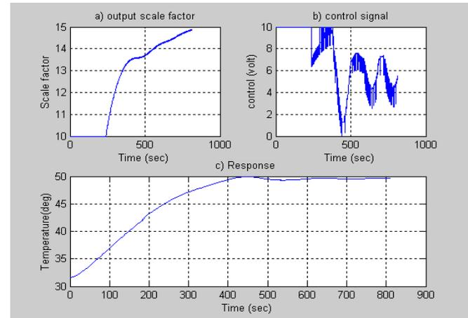
Fig. 16 Actual response using GD method in case of  $\alpha=0.5$  and initial gain = 10
