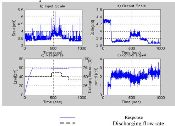
Fig. 27 Level response for step 60 cm and disturbed discharging flow rate
