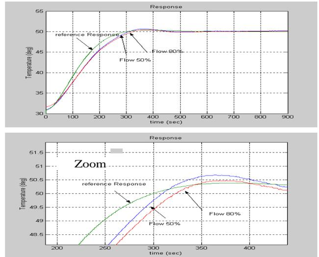
Fig. 25 Comparison between responses at 50% and 80% flow rate
