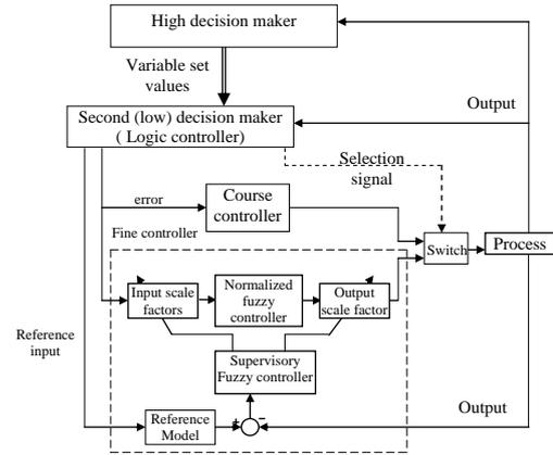
Fig. 6 Over-all block diagram of self adapted supervisory fuzzy
