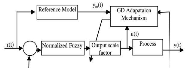
Fig. 4 Block diagram of GD adaptation system
