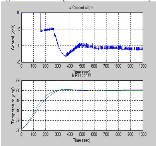
Fig. 23 Actual response using model reference supervisor controller at flow 50%
