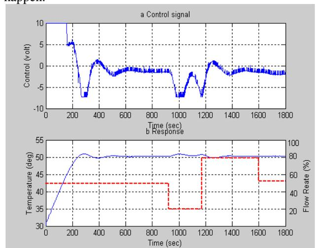
Fig. 21 Actual response using supervisor controller for input and output
