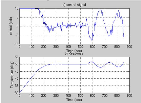
Fig. 10 Tuned PID response with disturbance effect
