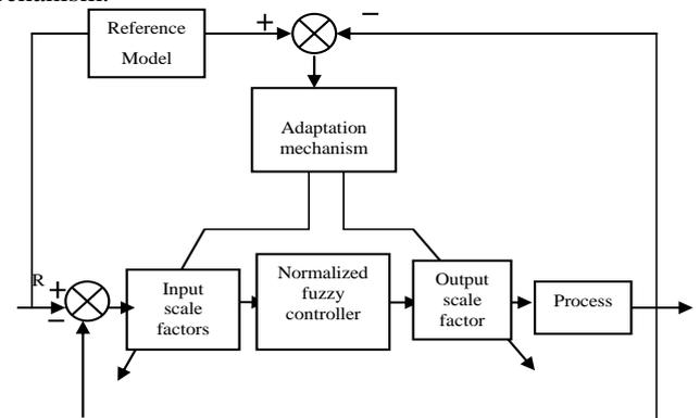
Fig. 1 General adaptation mechanism of Normalized fuzzy controller
