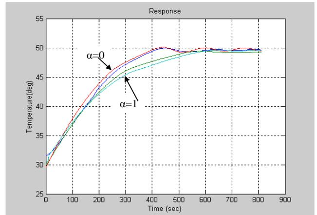
Fig. 17 Different responses for different values of  $\alpha$  at gain = 10
