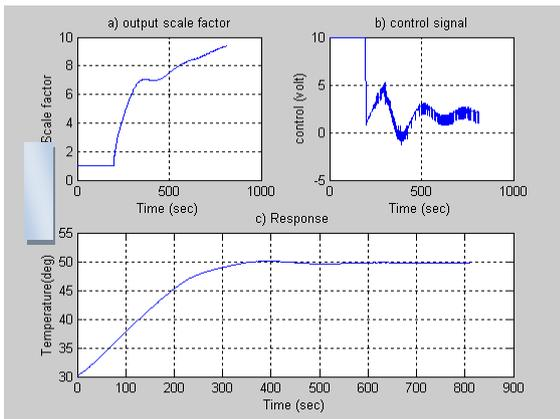
Fig. 14 actual response using GD method in case of  $\alpha=0.5$  and initial gain = 1
