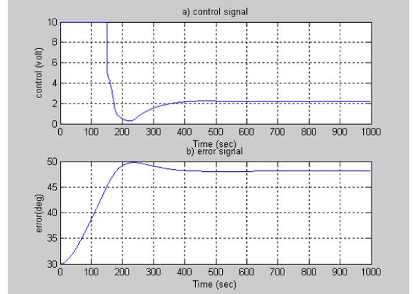
Fig. 11 simulation of normalized FLC
