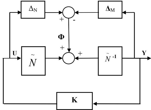
Fig. 1. Robust stabilization with respect to coprime factor uncertainty
