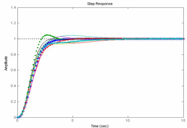
FIG ( 8 ) the system response due to Variation of parameters in case of using the PID weighting function in the H- inf synthesis
