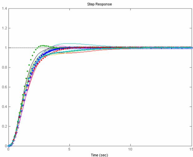
Fig( 7 ) the system response due to Variation of parameters in case of using the MOI weighting function in the H- inf loop shaping
