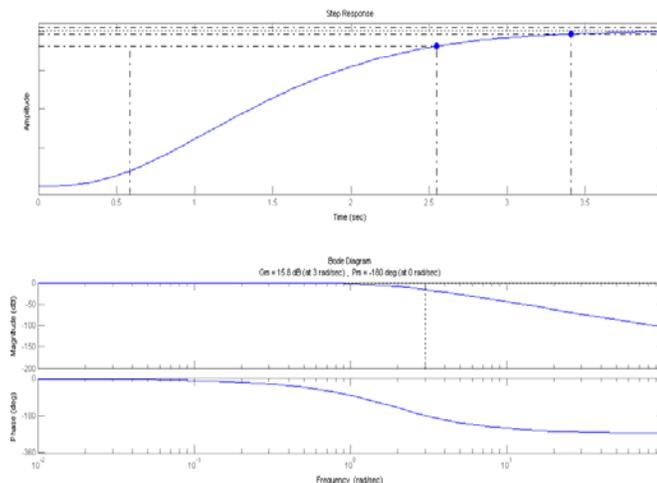
FIG ( 3 ) The system response due to step input in case of using the MOI weighting function for  $H_\infty$  loop shaping
