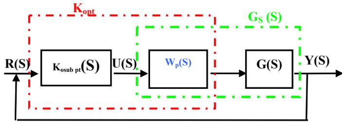
Fig(2) The standard H-∞ loop shaping closed loop system
