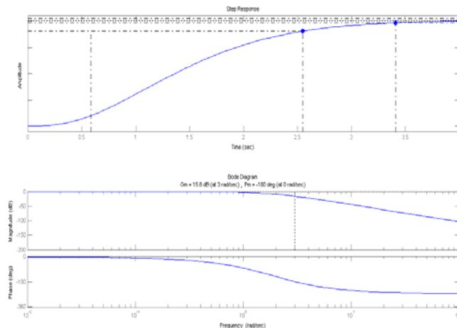
FIG ( 4 ) The system response due to step input in case of using the PID weighting function for  $H_\infty$  synthesis
