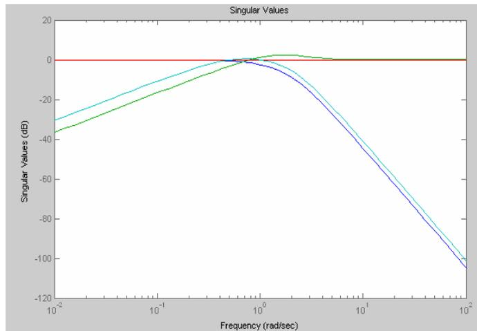
Fig(6) The singular value of  $\sigma(T)$  the complementary sensitivity,  $\sigma(S)$  is the sensitivity,  $\sigma(Su)$  the control sensitivity,  $\sigma(So)$  the output sensitivity(Si) input disturbances sensitivity,  $\sigma(r)=\sigma(T+Si)$ , in case of using a PID weighting function for H-  $\infty$  synthesis
