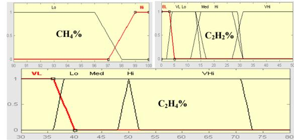
Figure 6. Duval fuzzy inputs with trapezoidal membership functions for gases ratio codes CH<sub>4</sub>%, C<sub>2</sub>H<sub>2</sub>% and C<sub>2</sub>H<sub>4</sub>%.
