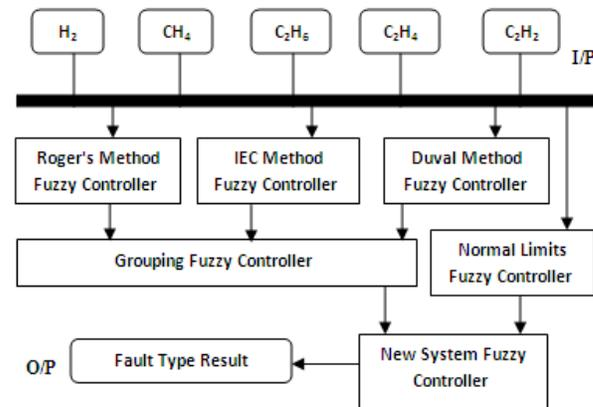
Figure 7. New fuzzy system technique block diagram.
