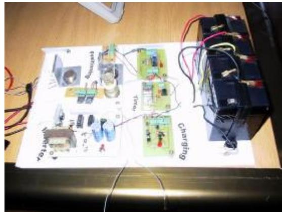
Figure (12) Sun tracking control circuit.
