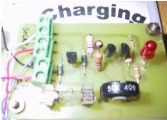
Figure (11) shunt regulator battery charging circuit photo.
