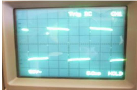
Figure (12) Inverter output voltage response.
