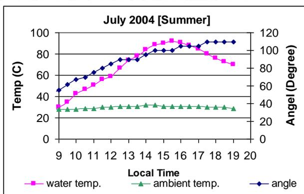
Fig. (4) Experimental test results for a summer clear day.
