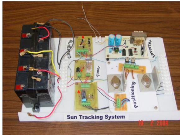
Fig. 1 The solar cooker with sun tracking system Fig. 2. Sun tracking control circuit.
