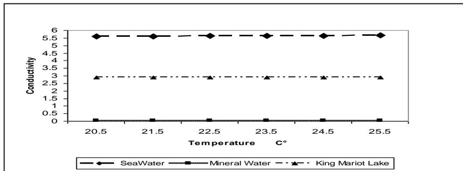
Fig 3- The comparison between average values of conductivity and temperature among three different sources of water
