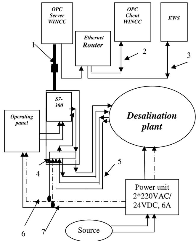
Figure (1) The desalination plant with SCADA system
