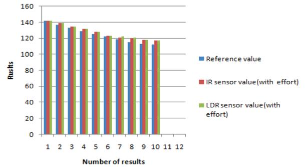
Figure 9. The comparison between the (HEM-907XL) results, the designed IR sensor results and the LDR sensor results for measuring heart beat rate (with effort).
