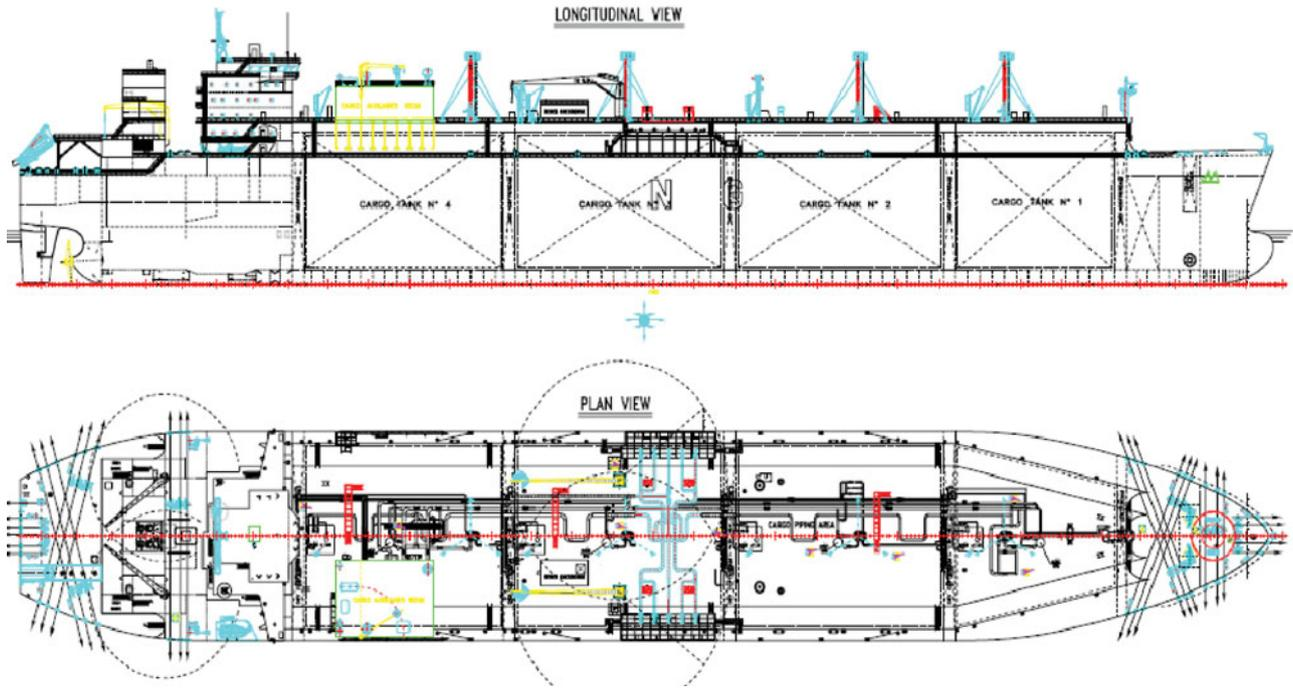
Figure 1. Principal particulars of the 138,000 m<sup>3</sup> LNG carrier (Safedor 2005). This figure is available in colour online.
