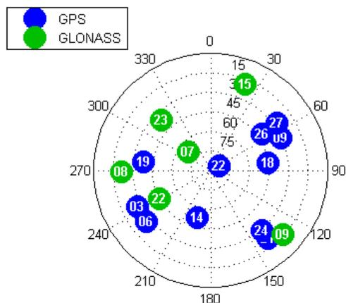
**Figure 5: Skyplot for the start of the WH test**
