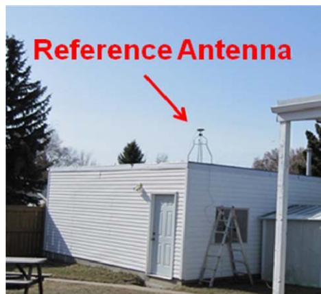
**Figure 3: Location of reference antenna for the WH test**
