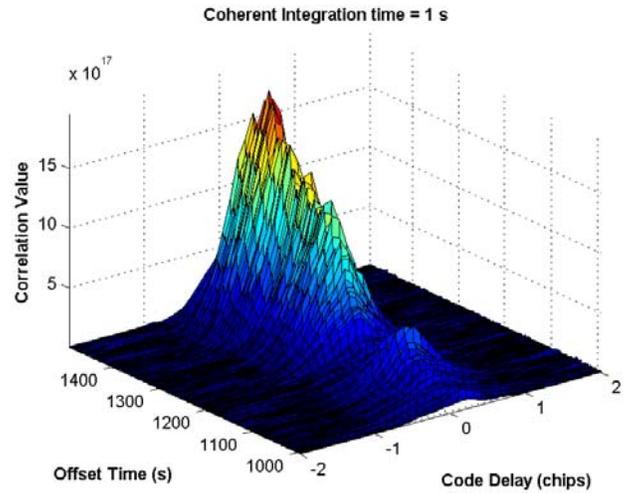
**Figure 18: Time series of correlator outputs for GPS PRN 27: 1 second coherent integration time**
