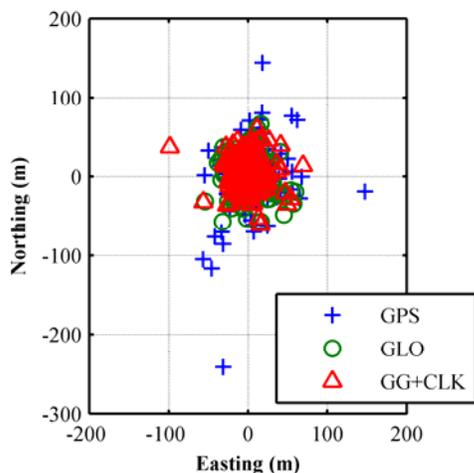
**Figure 23: Scatter plot of horizontal position errors computed for the NavLab test, using all measurements with  $C/N_0$  above 10 dB-Hz**
