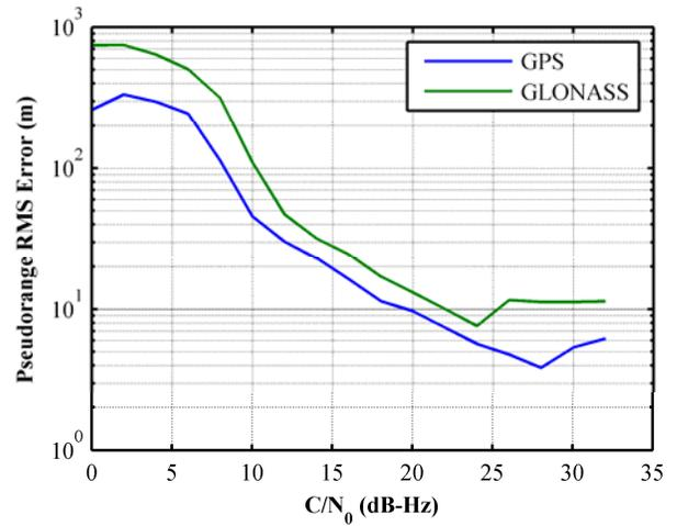
Figure 22: RMS pseudorange error vs receiver sensitivity for the NavLab test
