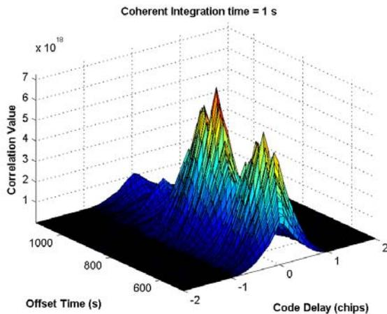
**Figure 7: Time series of correlator outputs for GLONASS PRN 9: 1 second coherent integration time**
