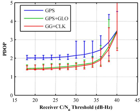
**Figure 13: Mean, max and min PDOP vs receiver sensitivity for the WH test. The continuous lines represent the mean value, the error bars report the maximum and minimum**
