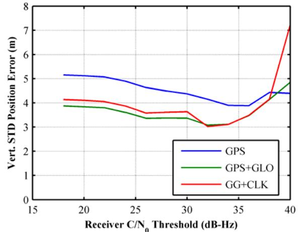
**Figure 15: Standard deviation of the vertical positions vs receiver sensitivity for the WH test**
