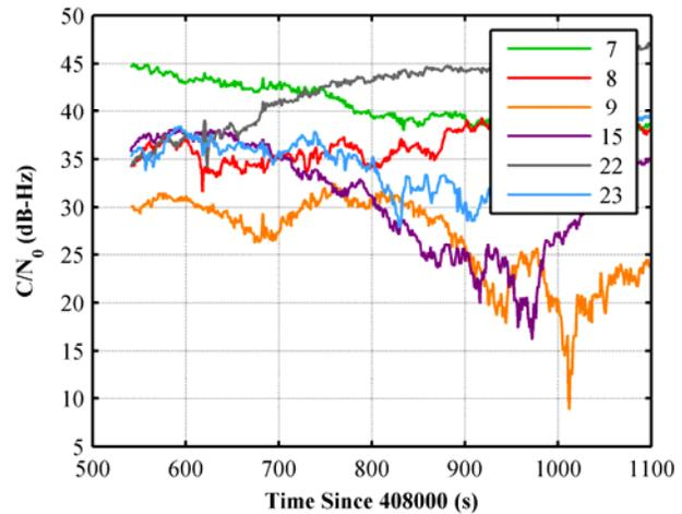
**Figure 9: Carrier-to-noise density ratio of the GLONASS signal received on the main floor of the WH.**
