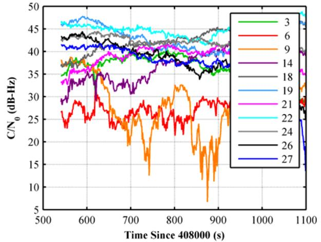
**Figure 8: Carrier-to-noise density ratio of the GPS signal received on the main floor of the WH.**
