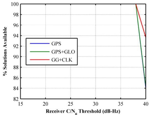
**Figure 12: Percentage solution availability vs receiver sensitivity for the WH test. Note that 100 % availability is seen in most cases**
