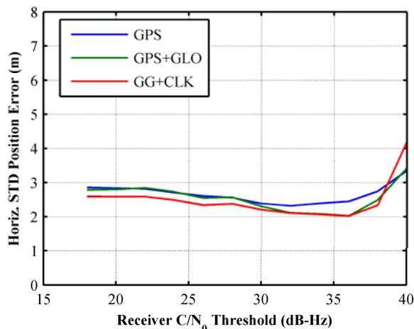
**Figure 14: Standard deviation of the horizontal positions vs receiver sensitivity for the WH test**
