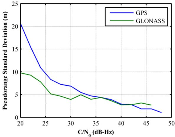
**Figure 10: Delta pseudorange standard deviations vs  $C/N_0$  for the WH test**
