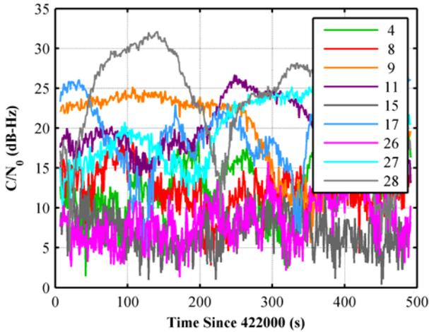
Figure 20: GPS  $C/N_0$  vs time for the NavLab test
