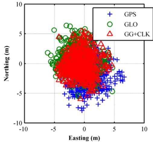
**Figure 11: Scatter plot of horizontal positions computed for the WH test. The origin is given by the mean value of the GG+CLK case**
