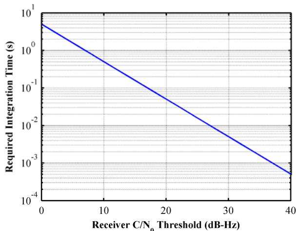
**Figure 28: Required integration time vs receiver C/N<sub>0</sub> threshold**
