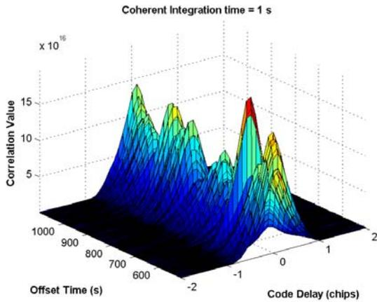
**Figure 6: Time series of correlator outputs for GPS PRN 6: 1 second coherent integration time**
