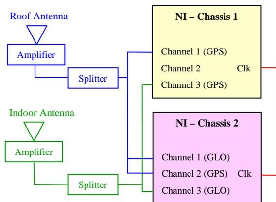
**Figure 2: Test setup adopted for collecting synchronous live GPS/GLONASS L1 C/A signals.**
