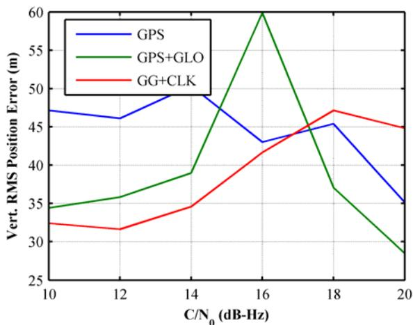
**Figure 27: Vertical RMS position error vs receiver sensitivity for the NavLab test**
