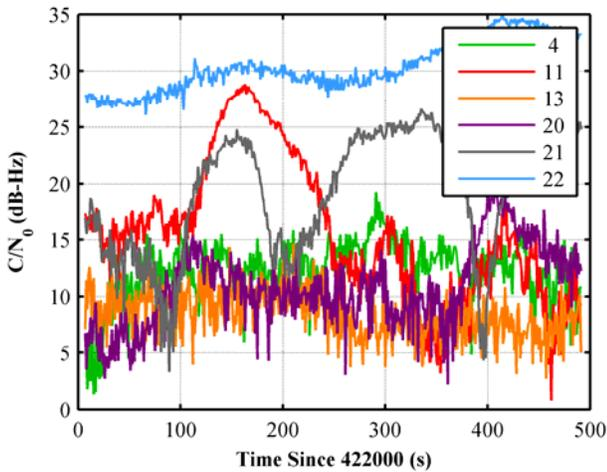
Figure 21: GLONASS  $C/N_0$  vs time for the NavLab test
