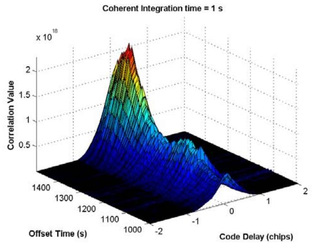
**Figure 19: Time series of correlator outputs for GLONASS PRN 22: 1 second coherent integration time**
