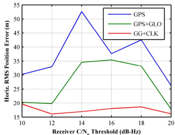
**Figure 26: Horizontal RMS position error vs receiver sensitivity for the NavLab test**
