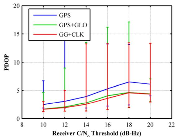
**Figure 25: Mean, max and min PDOP values vs receiver sensitivity for the NavLab test. The continuous lines represent the mean value, the error bars report the maximum and minimum**
