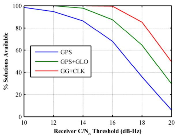
**Figure 24: Percentage availability of position solutions vs receiver sensitivity for the NavLab test**
