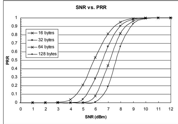
Fig. 3. SNR vs. PRR for Different Packet Lengths
