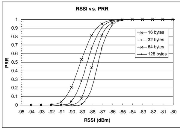
Fig. 4. RSSI vs. PRR for Different Packet Sizes
