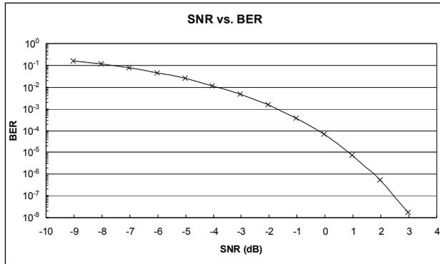
Fig. 2. SNR vs. BER for Zigbee at 2.4 GHz
