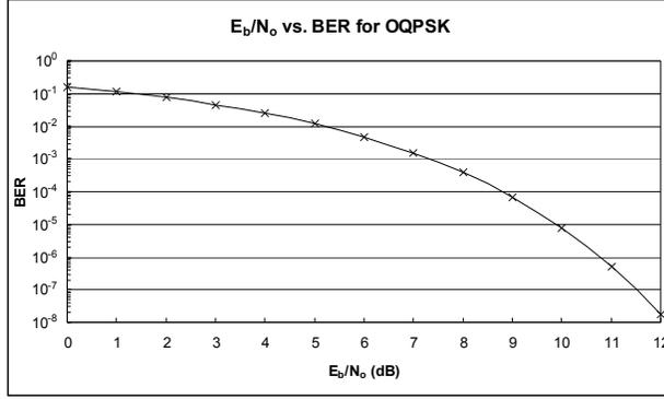
Fig. 1. Eb/No vs. BER for OQPSK Modulation
