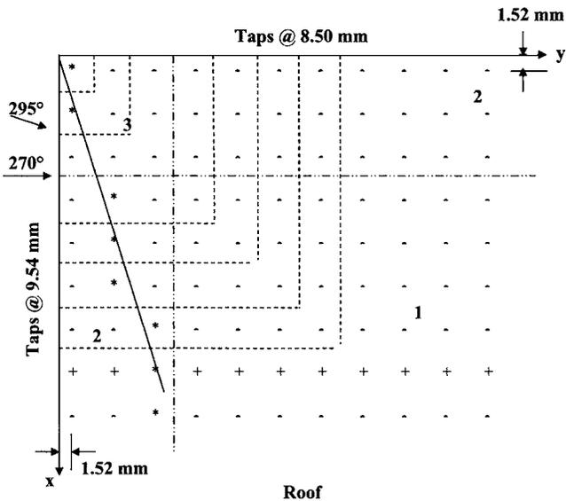
Fig. 1. Layout of roof pressure taps near roof corner with tributary zones
