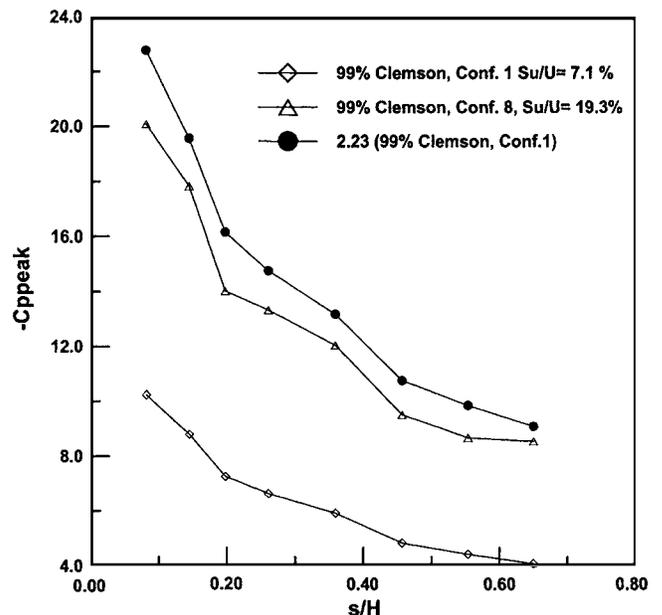
Fig. 14. Peak pressure coefficients of pressure tap Set B
