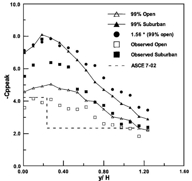
Fig. 2. Peak pressure coefficients distribution for Set I
