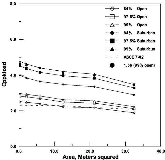
Fig. 11. Peak load coefficients for tributary areas of Fig. 9 with azimuth 295° (zone of positive mean pressure)
