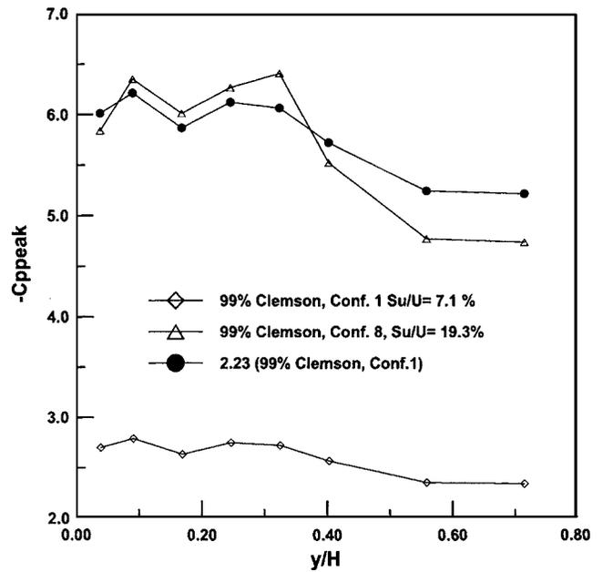
Fig. 13. Peak pressure coefficients for pressure tap Set A
