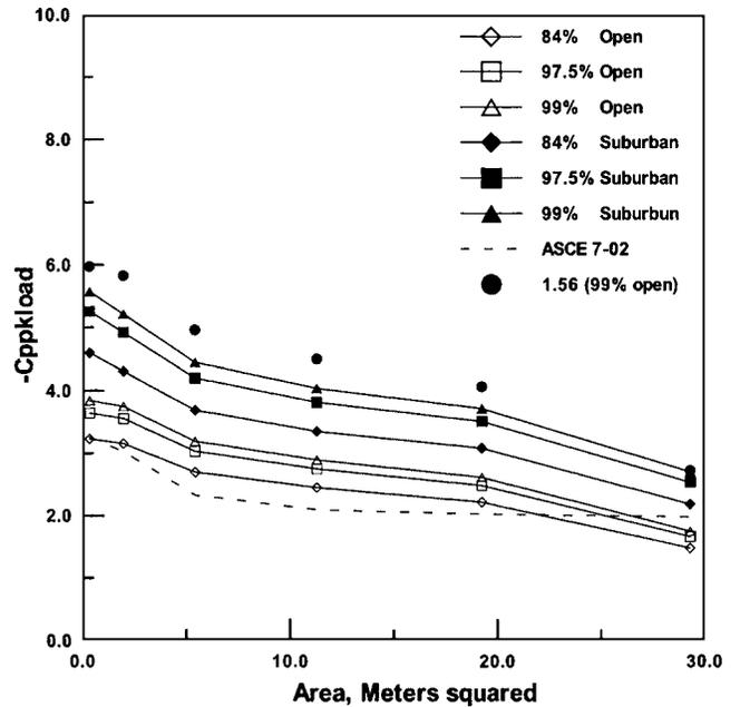
Fig. 10. Peak load coefficients for tributary areas of Fig. 9 with azimuth 270° (zone of flow separation)
