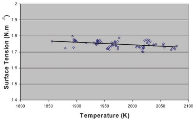
8 Surface tension of alloy IN718 as function of temperature<sup>17</sup>
