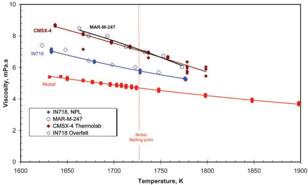
7 Viscosity of alloy IN 718, CMSX-4, MAR-M-247 and pure Ni as function of temperature; open symbols IN 718 and MAR-M-247 due to Overfelt *et al.*<sup>16</sup>
