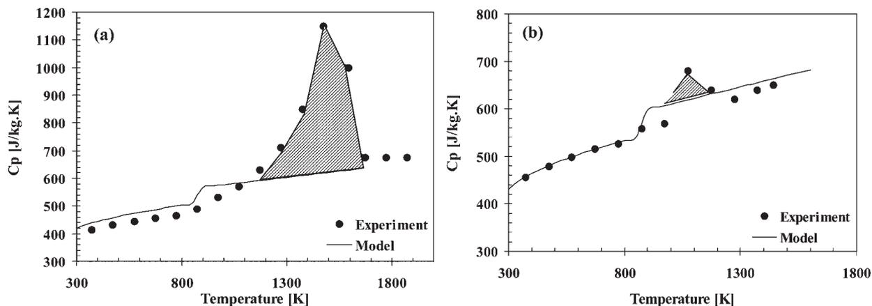
1 Heat capacity as function of temperature for a CMSX-4 and b IN718 showing method by which  $\Delta H^{fus}$  was obtained<sup>14</sup>
