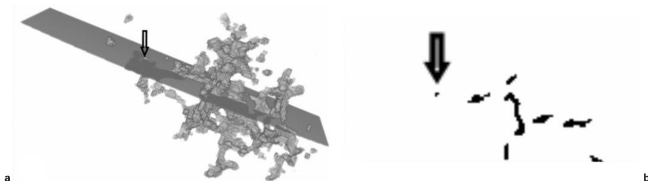
4 Comparison of a 3D pore morphology with that observed on b 2D section
