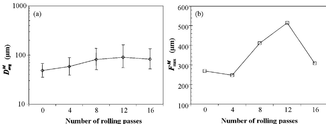
7 Metallographically quantified a mean equivalent pore diameter  $D_{\text{avg}}^{\text{M}}$  and b maximum Feret length  $F_{\text{max}}^{\text{M}}$  as function of number of rolling passes for Al-6Mg alloy after H10
