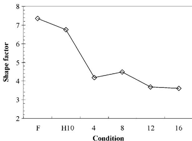
9 Shape factor evolution as function of homogenisation and number of rolling passes for Al-6Mg alloy (XMT): numbers indicate rolling passes
