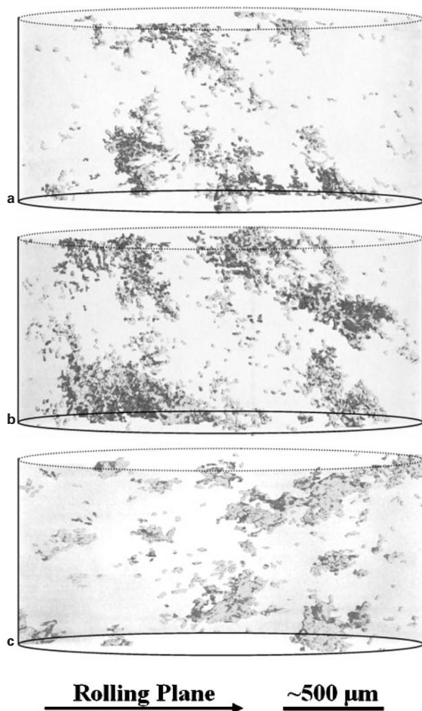
6 X-ray microtomography rendering of porosity in larger volume of Al-6Mg for a F, b H10 and c after 12 rolling passes
