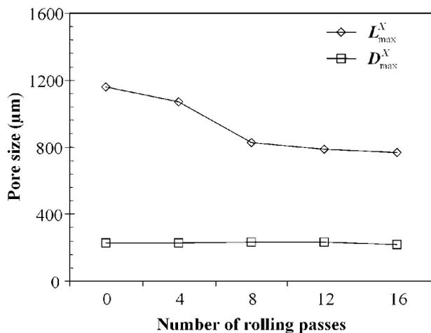
8 X-ray microtomography quantified maximum equivalent pore diameter  $D_{max}^X$  and maximum pore length  $L_{max}^X$  as function of number of rolling passes for Al-6Mg alloy after H10
