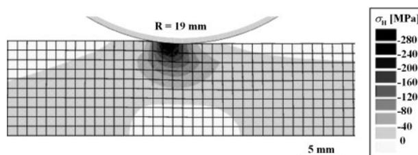
10 Hydrostatic stress  $\sigma_H$  distribution during plane strain rolling of 20 mm thick plate with roll radii  $R$  of 19 mm
