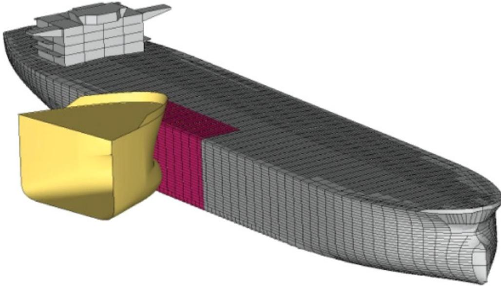
Figure 8. Example of a finite element simulation of a ship–ship collision. (This figure is available in colour online.)
