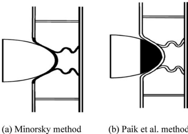
Figure 9. Method to calculate the damage volume of the struck ship structure (Paik et al. 1999).
