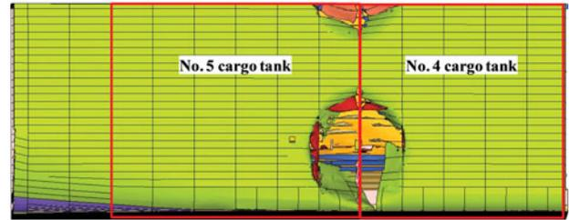
Figure 11. Scenario 18 result involving the rupture of two cargo tanks. (This figure is available in colour online.)
