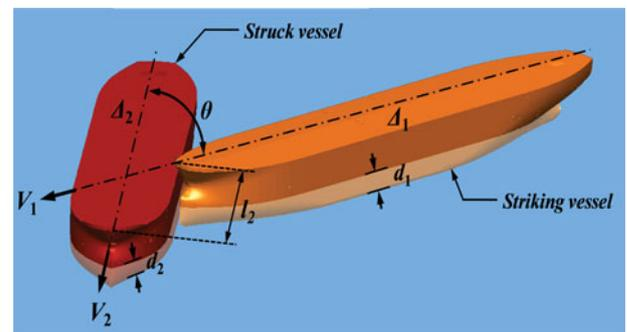
Figure 7. Schematic of a ship-ship collision. (This figure is available in colour online.)
