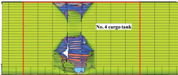
Figure 10. Scenario 15 result involving the rupture of one cargo tank. (This figure is available in colour online.)
