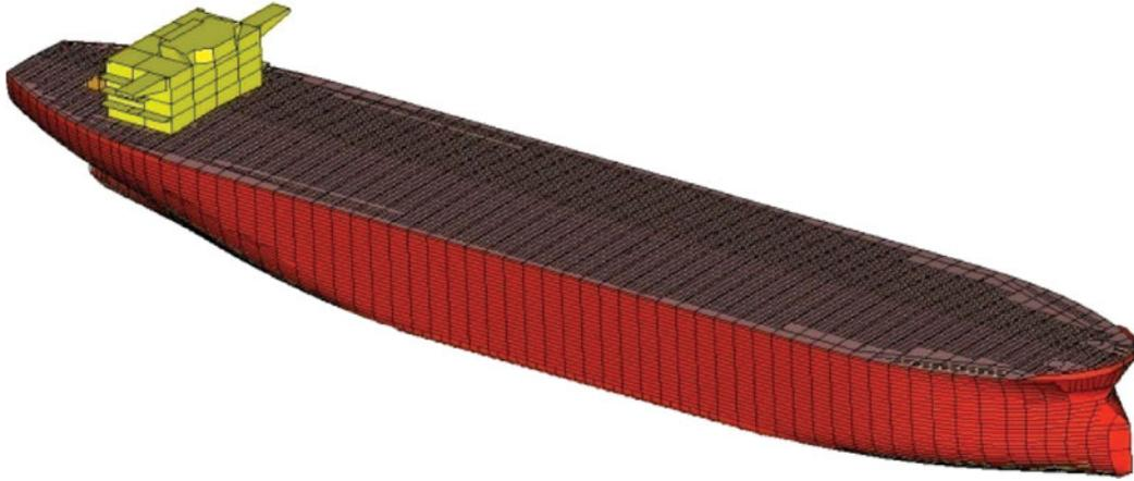
Figure 4. Geometric model of the struck ship. (This figure is available in colour online.)
