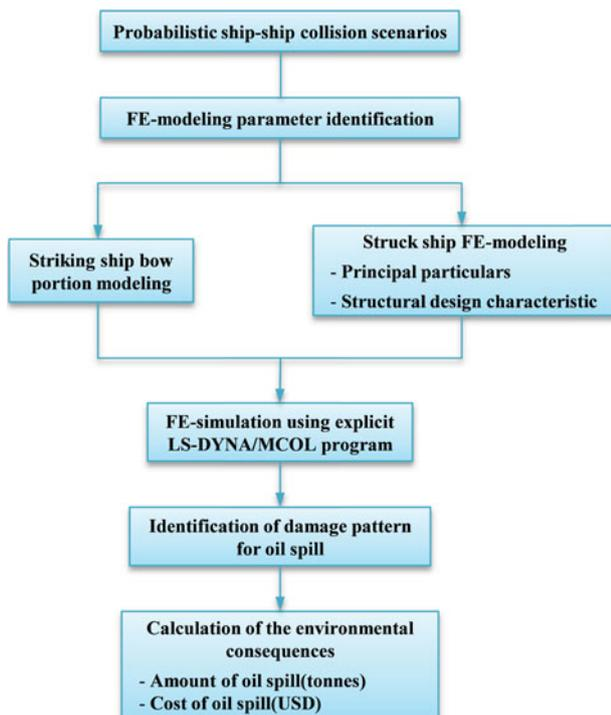
Figure 3. Collision involved oil spill assessment procedure. (This figure is available in colour online.)
