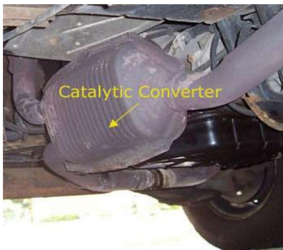
Fig. 3: Catalytic converter mounted in a car's exhaust system. (Source: Courtesy Wikimedia Commons, Public Domain).
