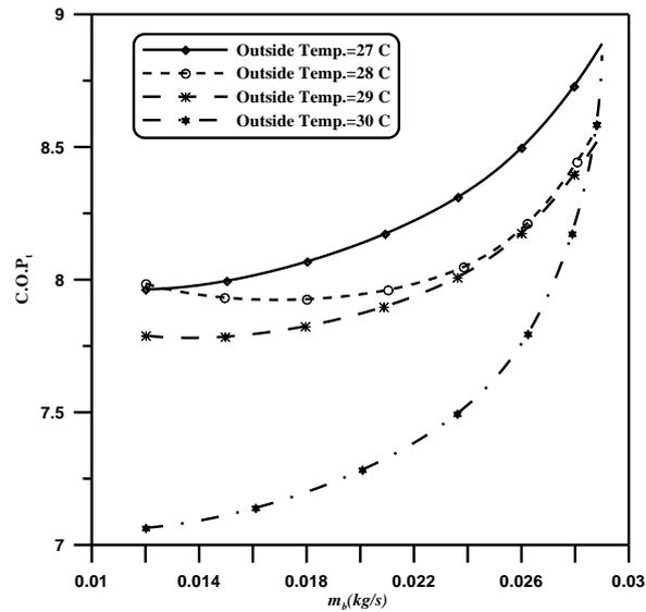
Fig.18: Effect of bled mass flow vers. C.O.P at room temp. of 24 oC
