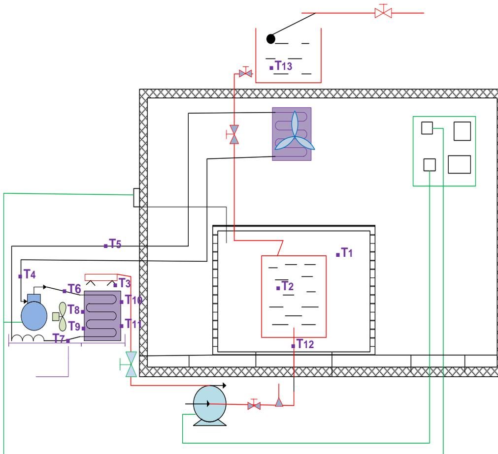
**Fig.2: Thermocouples Distribution in the System**
