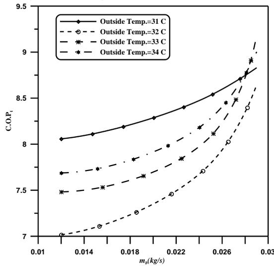
Fig.13: Effect of bled mass flow versus C.O.P at room temp. of 18 oC
