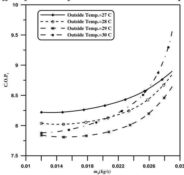
Fig.16: Effect of bled mass flow vers. C.O.P at room temp. of 22 oC
