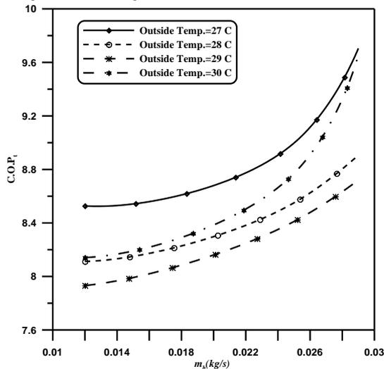
Fig.14: Effect of bled mass flow vers. C.O.P at room temp. of 20 oC
