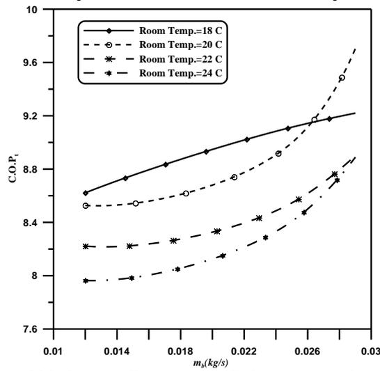
Fig.4: Effect of bled mass flow versus C.O.P at outside temp. of 27 °C
