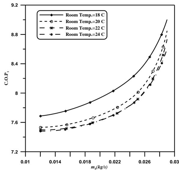
Fig.11: Effect of bled mass flow vers. C.O.P at outside temp. of 34 °C
