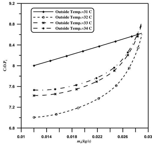
Fig.15: Effect of bled mass flow versus C.O.P at room temp. of 20 oC
