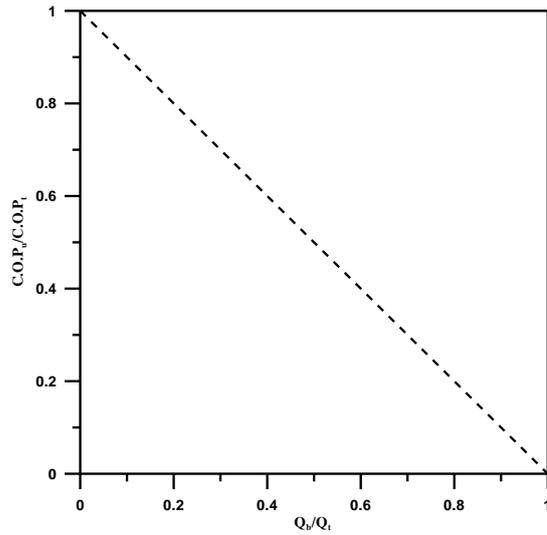
Fig.3: The useful C.O.P versus the amount of extracted heat Q<sub>b</sub>
