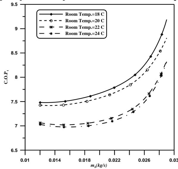
Fig.10: Effect of bled mass flow vers. C.O.P at outside temp. of 33 °C
