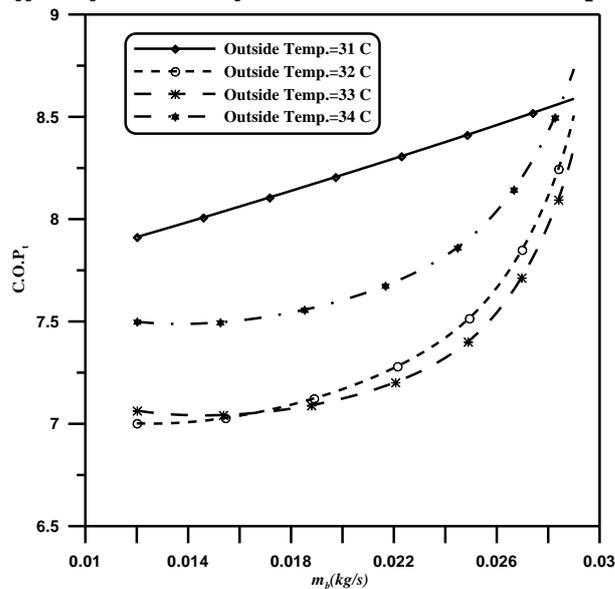
Fig.17: Effect of bled mass flow versus C.O.P at room temp. of 22 oC
