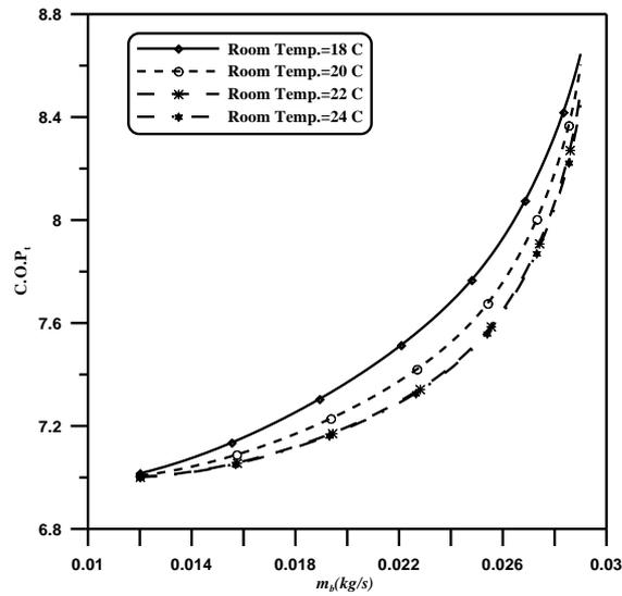
Fig.9: Effect of bled mass flow vers. C.O.P at outside temp. of 32 °C
