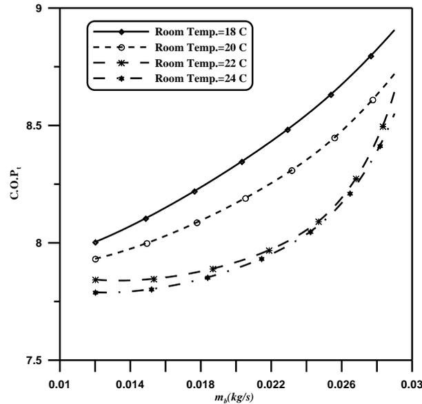
Fig.6: Effect of bled mass flow vers. C.O.P at outside temp. of 29 °C
