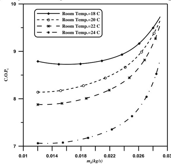
Fig.7: Effect of bled mass flow vers. C.O.P at outside temp. of 30 °C
