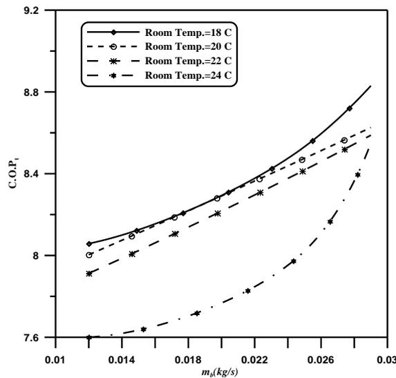
Fig.8: Effect of bled mass flow vers. C.O.P at outside temp. of 31 °C
