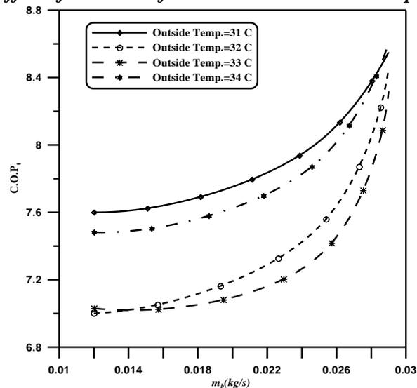
Fig.19: Effect of bled mass flow versus C.O.P at room temp. of 24 oC
