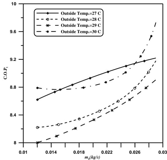
Fig.12: Effect of bled mass flow vers. C.O.P at room temp. of 18 oC
