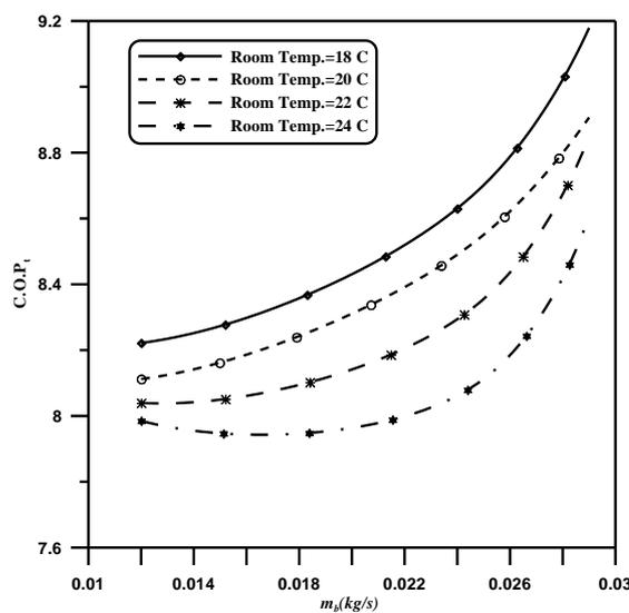
Fig.5: Effect of bled mass flow versus C.O.P at outside temp. of 28 °C
