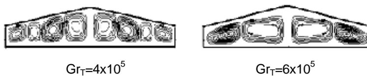
**Figure 13:** Streamlines  $Le=1$ ,  $N=1$  and  $\phi=10^\circ$ .
