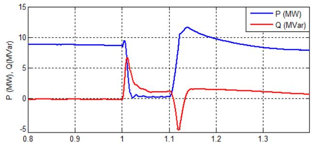
Fig. 5. Active power and reactive power fed to PCC from the wind farm.
