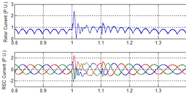
Fig. 6. The peak rotor current and the three-phase RSC current.
