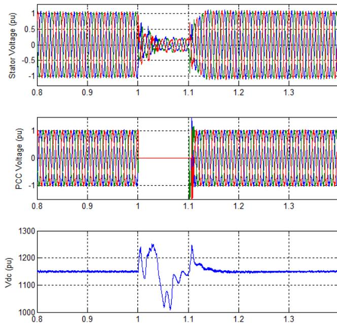
Fig. 7. The stator voltage, the PCC voltage, and the dc-link voltage.
