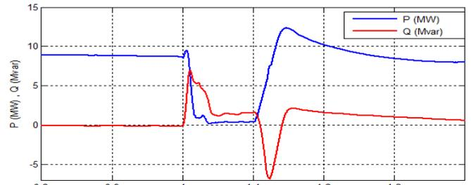
Fig. 8. Active power and reactive power fed to PCC from the wind farm.
