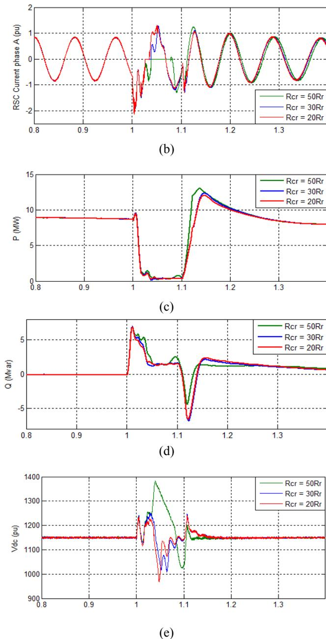
Fig. 10. Effect of varying crowbar resistance on the dynamic performance of the DFIG.
