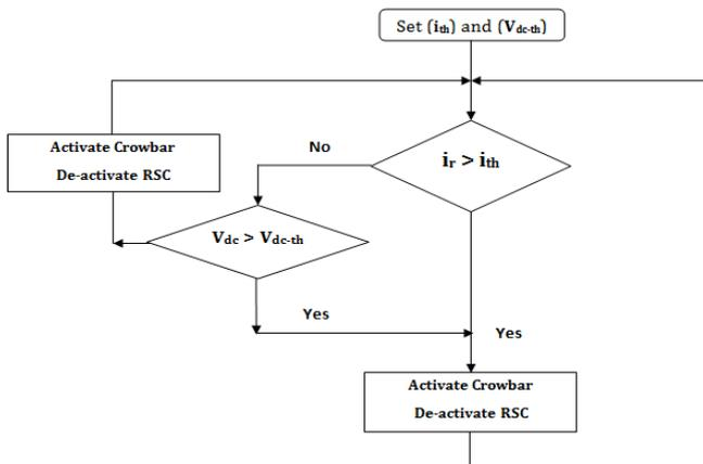
Fig. 3. Active crowbar control flowchart
