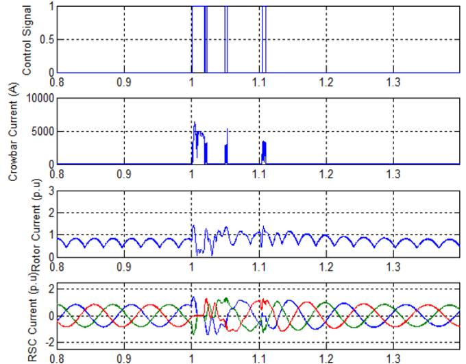
Fig. 9. Control signal, crowbar current, the peak rotor current, and the three-phase RSC Current.
