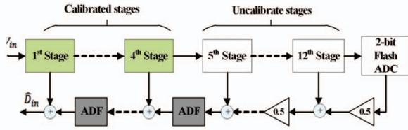
Fig. 3. The proposed calibration technique
