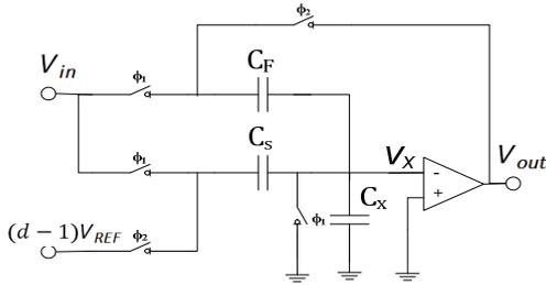
Fig. 2. 1.5 bit/stage MDAC architecture
