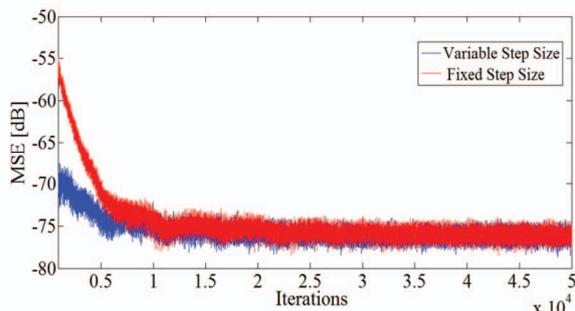
Fig. 6. Learning curve of variable step size vs fixed step size
