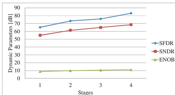
Fig. 5. Dynamic parameters vs stages calibrated
