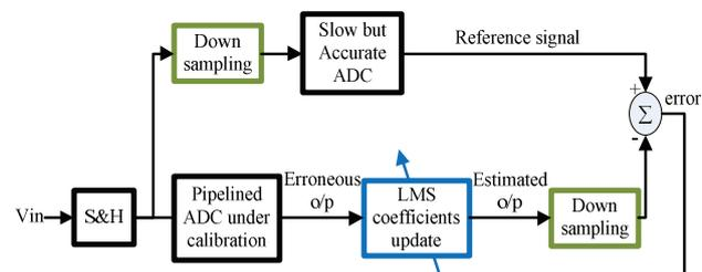
Fig. 1. Background calibration using parallel slow but accurate ADC
