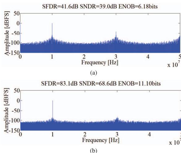
Fig. 7. Frequency spectrum at  $f_s=100$  Msample/s and  $f_{in}=9.99$  MHz (a) before calibration, (b) after calibration
