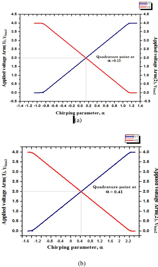
Fig.6 The relation between the input bias voltage and the parameter- $\alpha$ . (a) While using Bessel filter (b) without filtering.
