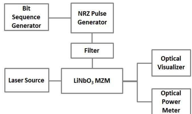
Fig. 2 Schematic diagram of the transmitter.
