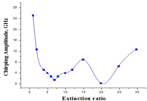
Fig. 7 Relation between the chirping amplitude and the extinction ratio.
