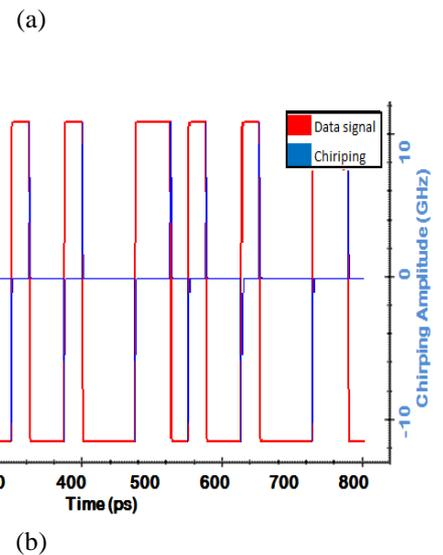
Fig.3 a) Input NRZ digital data signal. b) MZM output optical data with no filtering.
