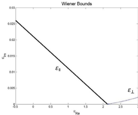
Figure 12: The Wiener bounds,  $\epsilon_{\parallel}$  and  $\epsilon_{\perp}$ , of a Silver-Silica layered composite.
