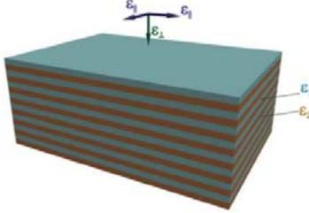
Figure 11: Schematic of a layered metal-dielectric structure, with the permittivities of the two constituents given as  $\epsilon_1$  and  $\epsilon_2$ , respectively. Two principal effective permittivities,  $\epsilon_{\parallel}$  and  $\epsilon_{\perp}$  [13].
