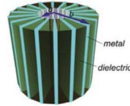
Figure 10: Schematic of a cylindrical non-magnetic cloak with high-order transformations for TM polarization [23].
