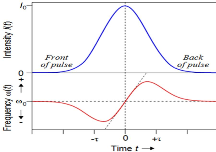
When an optical pulse is transmitted through an optical fiber, the Kerr effect causes a time-dependent phase shift according to the time-dependent pulse intensity. So SPM modulates the phase of the pulse by an amount proportional to the instantaneous pulse intensity [16, 17].
