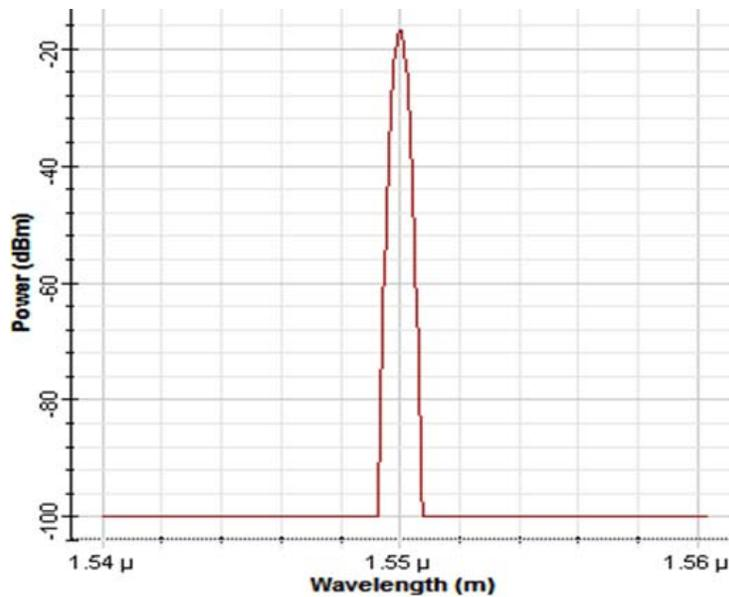
**Figure 4:** Broadening effect obtained due to SPM in DCF fiber of 100 m length with EDFA gain of 45 dB
