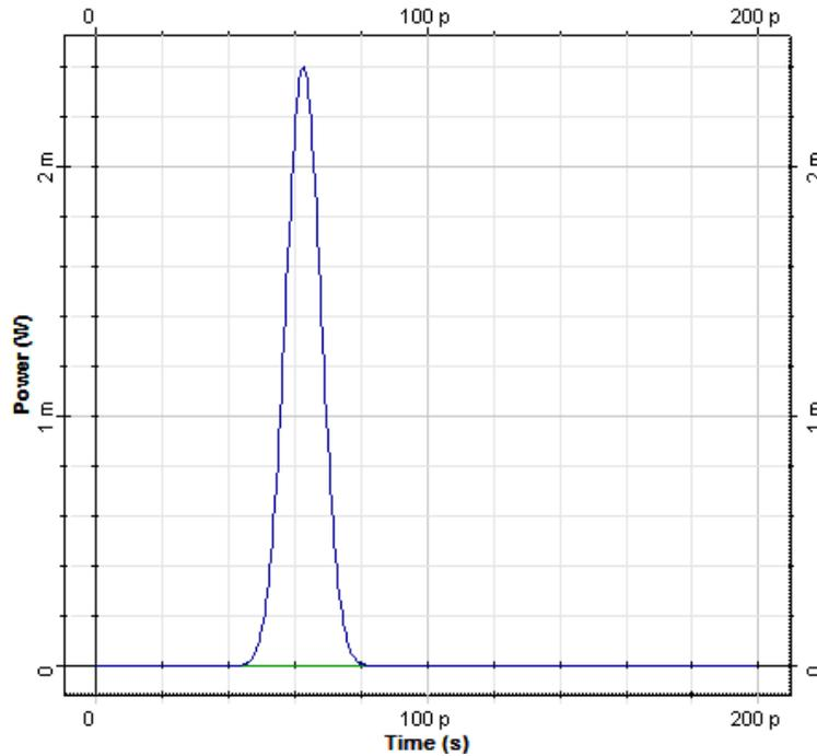
**Figure 7:** Converted optical pulse after the optical filter with central wavelength of 1555 nm
