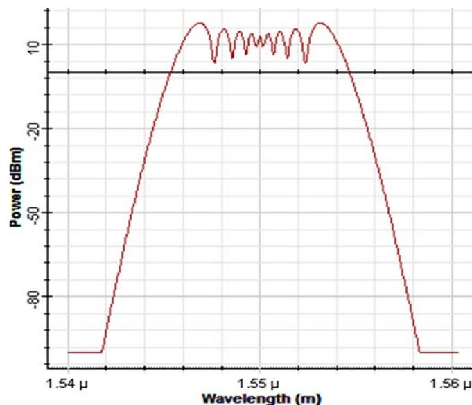
**Figure 5:** Converted spectrum obtained after the filter with central wavelength of 1555 nm
