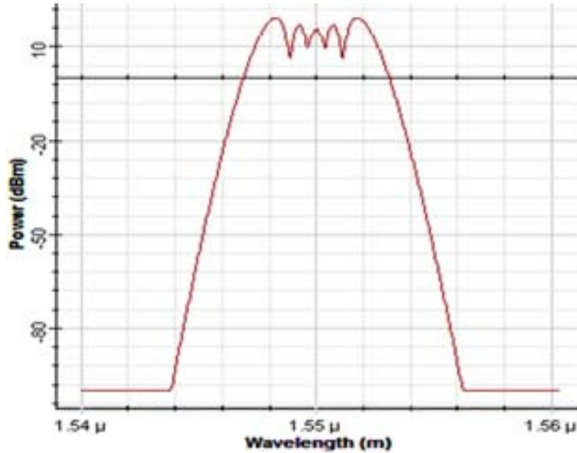
At the output of the system, a wavelength conversion is achieved with a good efficiency as shown in Fig.9 with a tunable optical filter with central wavelength of 1553.5 nm. The power peak is located at 1553.5 nm.
