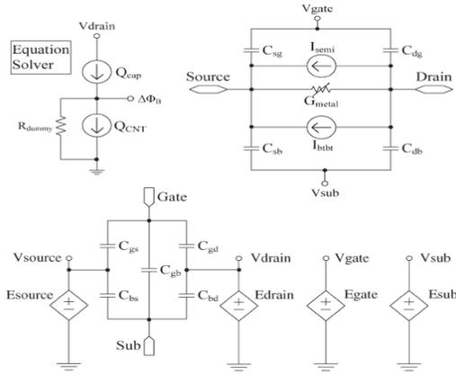
Fig. 1. Circuit model for the CNT [2].
