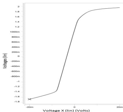
Fig 4. Transfer function (folded cascode CMOS 180nm)
