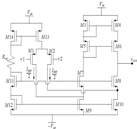
Fig 3. Folded Cascode Amplifier Circuit
