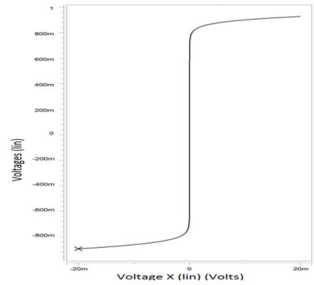
Fig 5. Transfer function (folded cascode CNFET 32nm)
