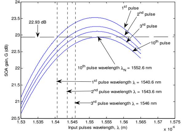
**Figure 2:** SOA gain response of a burst of Gaussian pulses against wavelength.
