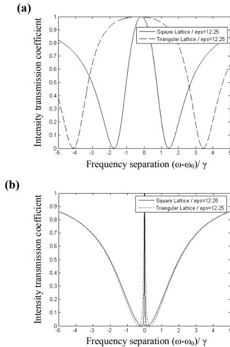
Fig. 2. Transmission spectra through the coupled resonator unit cell for two cases: a structure with square lattice, and a structure with a triangular lattice,  $\gamma$  is the decay rate of a given resonator.
