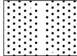
Fig. 1. Schematic of a two-dimensional triangular lattice photonic crystal structure with dielectric rods of radius  $0.2a$ . Removing one row of dielectric rods creates a waveguide. In each unit cell, two single-mode cavities are created on opposite sides of the waveguide with a separation  $l_i=7a$  [1]
