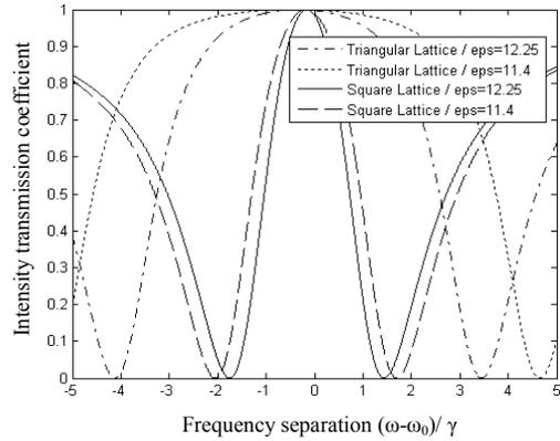
Fig. 4. Intensity transmission through different combinations of lattice geometry and dielectric constant investigated.
