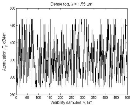
Fig. 10 Attenuation at  $\lambda=1.55 \mu\text{m}$  in dense fog.
