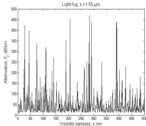
Fig. 8 Attenuation at  $\lambda=1.55 \mu\text{m}$  in light fog.
