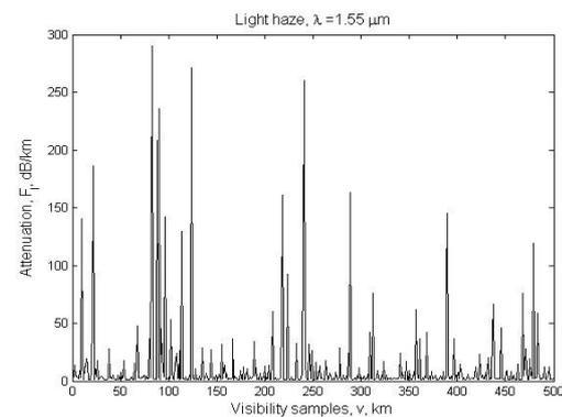
Fig. 5 Attenuation at  $\lambda=1.55 \mu\text{m}$  in light haze.
