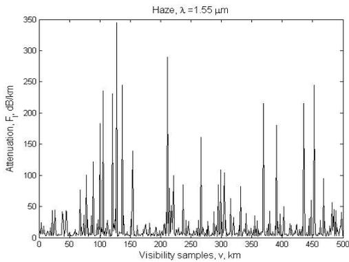
Fig. 6 Attenuation at  $\lambda=1.55 \mu\text{m}$  in haze weather.
