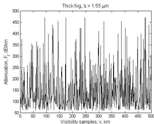
Fig. 9 Attenuation at  $\lambda=1.55 \mu\text{m}$  in thick fog.
