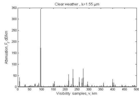
Fig. 4 Attenuation at  $\lambda=1.55 \mu\text{m}$  in clear weather.
