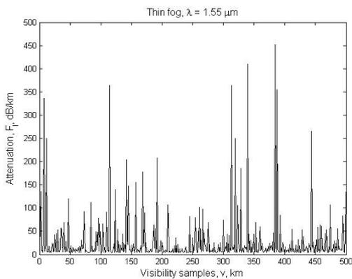
Fig. 7 Attenuation at  $\lambda=1.55 \mu\text{m}$  in thin fog.
