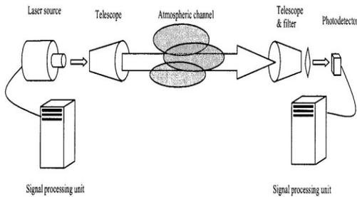
Fig. 2 Schematic structure of a WOC system.
