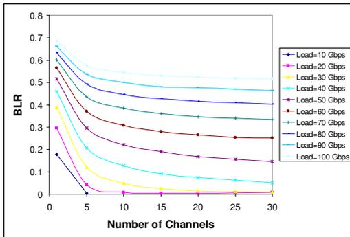
Fig. 5 Relation between BLR and number of channels at different load.
