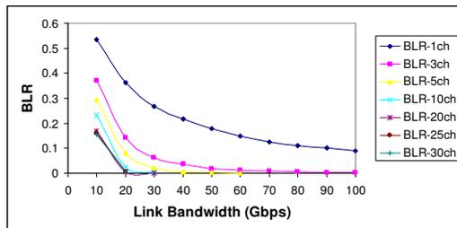
Fig. 8 BLR against link bandwidth at different number of channels.
