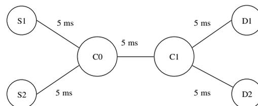
Fig. 2 OBS simulated network topology.
