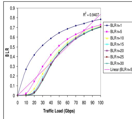
Fig. 3 Relation between BLR and traffic load different number of channels (n).
