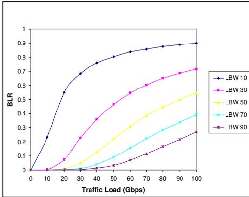
Fig. 4 Relation between BLR and traffic load for different number of link bandwidths (LBW).
