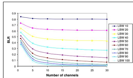
Fig. 6 Relation between BLR and number of channels at different link bandwidths.
