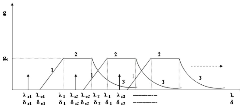
Figure 1 Gain,  $g$ , of multi-pump Raman amplifier.
