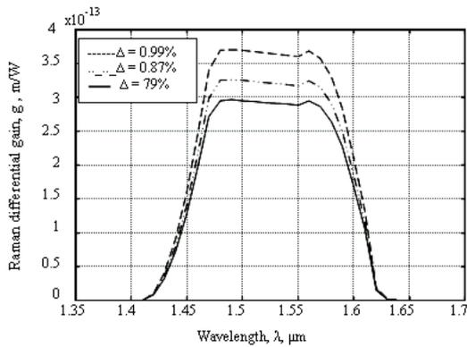
Figure 13 Variation of differential Raman gain with wavelength.
