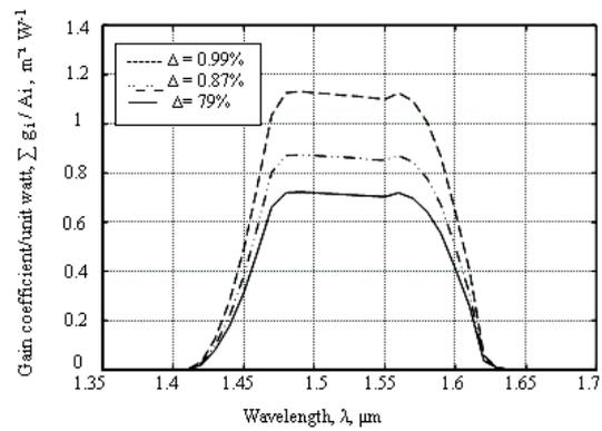
Figure 14 Gain coefficient per unit watt against wavelength.
