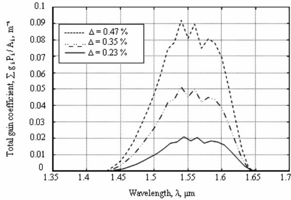
Figure 12 Variation of total gain coefficient with wavelength.
