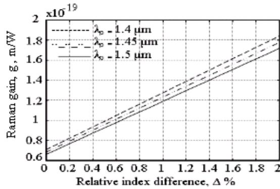
Figure 4 Raman gain versus relative refractive index difference.
