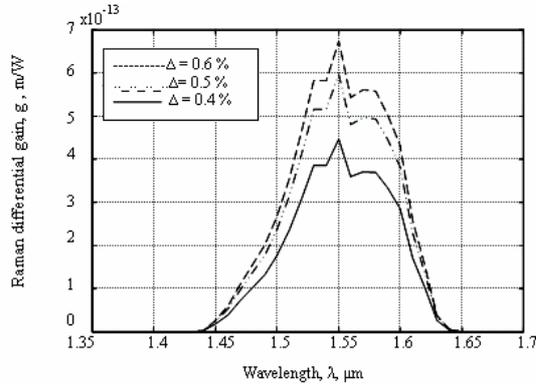
Figure 7 Differential Raman gain versus wavelength.
