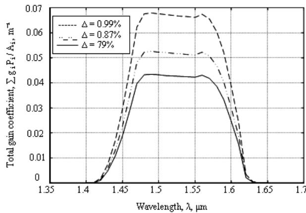
Figure 15 Variation of total gain coefficient with wavelength.
