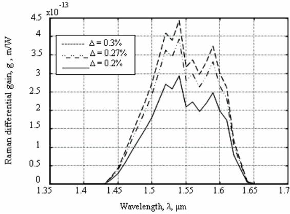
Figure 2 Variation of differential Raman gain with wavelength.
