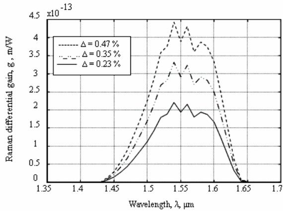
Figure 10 Variation of differential Raman gain with wavelength.
