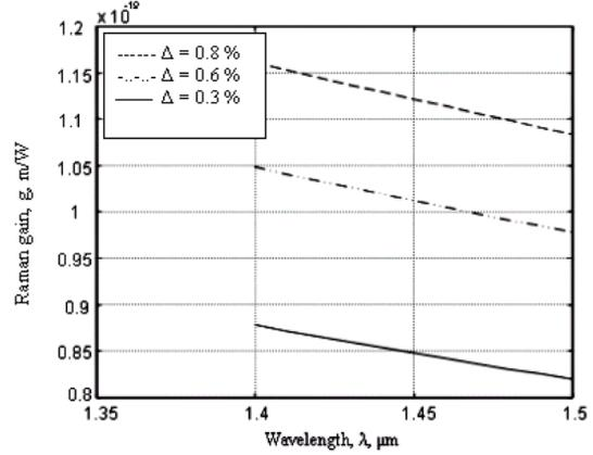
Figure 3 Raman gain against pumping wavelength.
