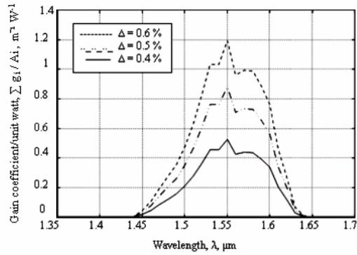
Figure 8 Gain coefficient per unit watt against wavelength.
