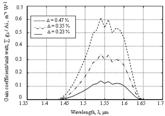
Figure 11 Gain coefficient per unit watt against wavelength.
