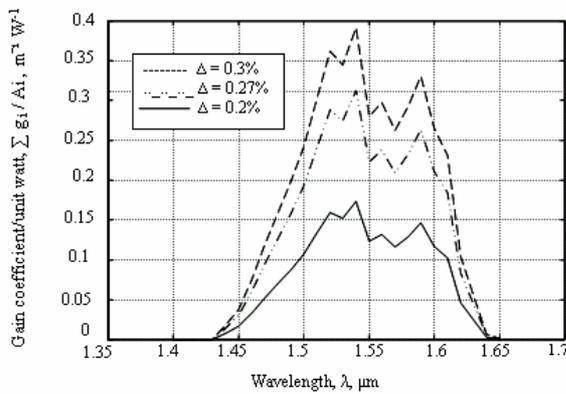
Figure 5 Gain coefficient per unit watt against wavelength.
