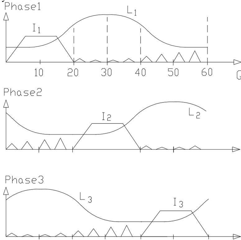
Fig. (10): Current waveforms of the 3-ph SRM
