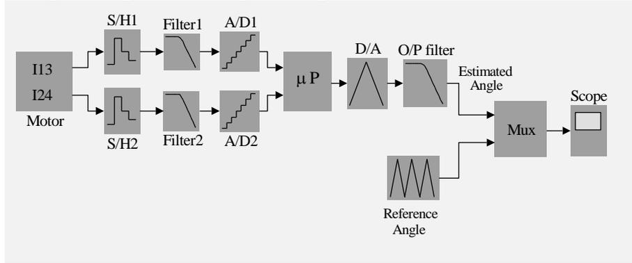
Fig. (5) Schematic diagram for the position detection circuit simulation
