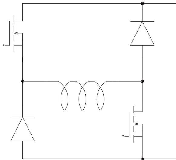
Fig. (4) Asymmetric half bridge converter per phase
