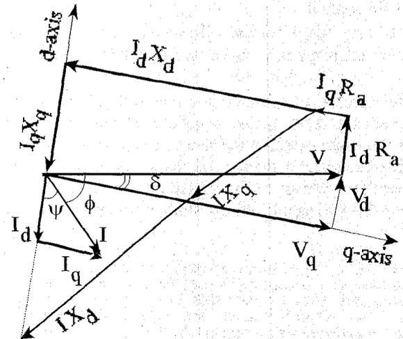
Fig. 2 Phasor diagram of three phase parametric motor
