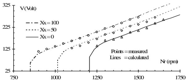
Fig. 5 Relation of no-load voltage and speed for different added series reactance
