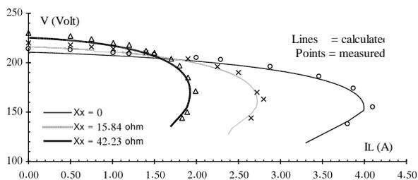
Fig. 6 Relation of load voltage and current for different series reactance
