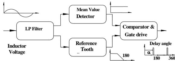
Fig. 10. The closed loop voltage control circuit
