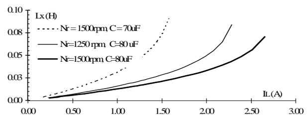
Fig. 8 Relation between load current and inductor needed to keep constant voltage.
