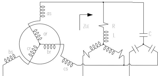
Fig. 1 Connection of SCSM
