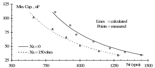
Fig. 7 Relation of minimum excitation capacitor and speed for different added series reactance
