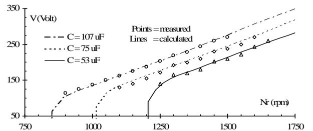
Fig. 3 Relation of no-load voltage and speed for different excitation capacitors
