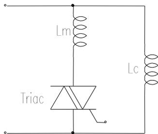
Fig. 9 Variable inductor circuit
