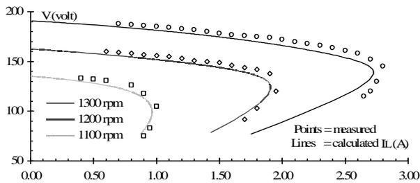
Fig. 4 Relation of load voltage and current at different speeds
