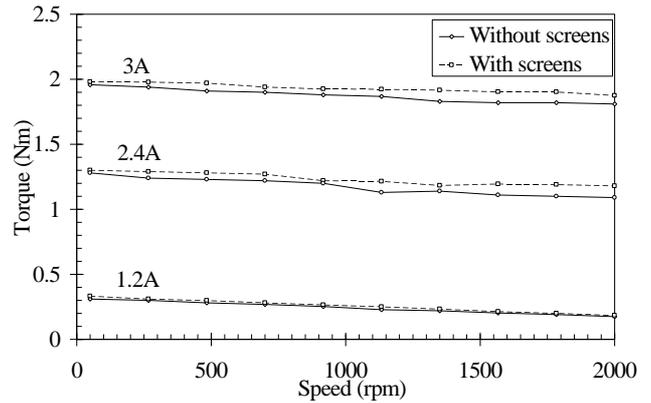
Fig. 9. Torque/Speed characteristics at different current levels for screened and non-screened 4-ph SRM rotors
