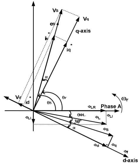
Fig. 2. Space vector diagram for UPFC of PMSM.
