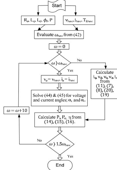
Fig. 4 Flow chart of the performance of vector control at steady-state.
