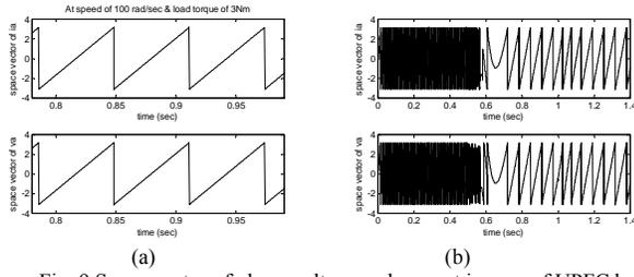
Fig. 9 Space vector of phase voltage and current in case of UPFC by controlling  $\theta_s$ : (a) At rated speed and torque, (b) At step change of speed and torque.
