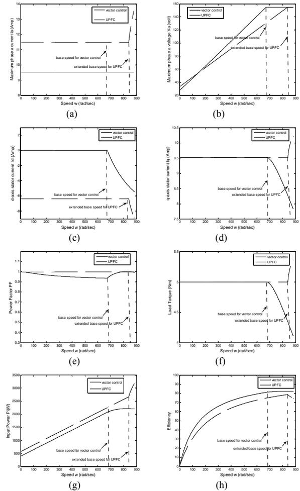
Fig. 6 Steady-state performances of both vector control & UPFC.
