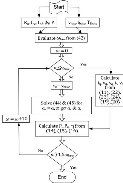
Fig. 5 Flow chart of the performance of UPFC at steady-state.
