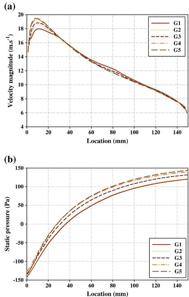
**Fig. 2.** Line (DE) grid-independency profiles of (a) velocity and (b) static pressure.
