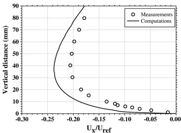
Fig. 4. Normalized computed Y velocity component in comparison with measurements.
