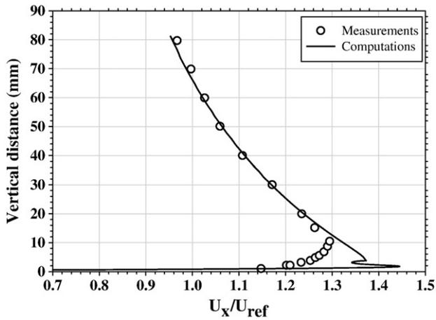
Fig. 3. Normalized computed X velocity component in comparison with measurements.
