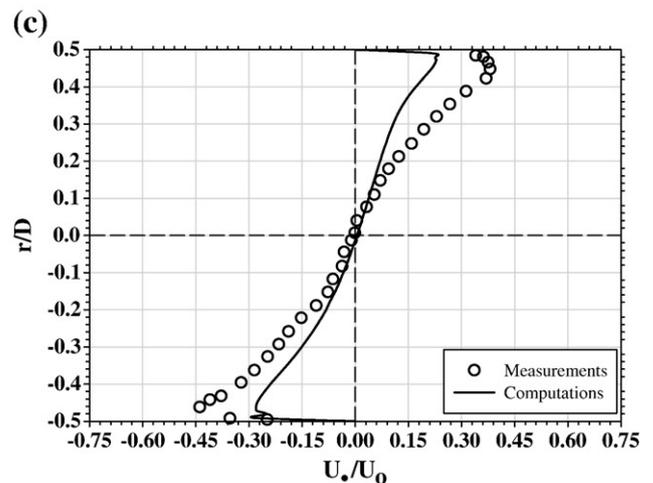
Fig. 5. Comparison between measured [19] and computed normalized tangential velocity along line BC in the cavity for (a)  $Re = 5.285 \times 10^4$  (b)  $Re = 9.155 \times 10^4$  and (c)  $Re = 1.302 \times 10^5$ .
