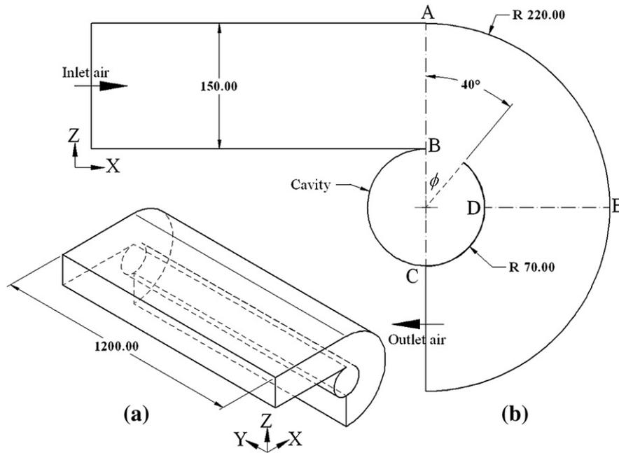
Fig. 1. Flow configuration in the open cylinder cavity after [19]. Dimensions in mm. (a) a schematic of the 3D flow configuration and (b) the 2D flow domain considered in the present study.
