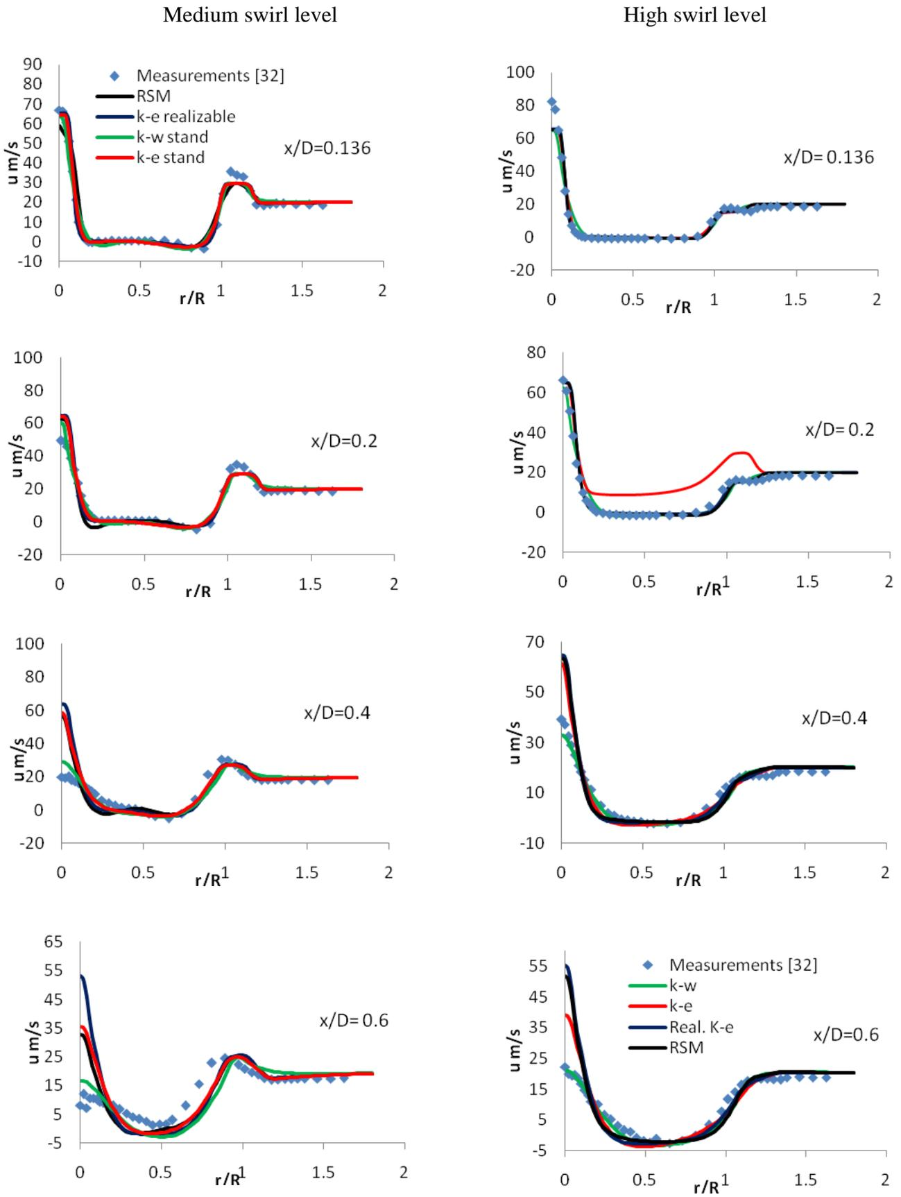
Figure 4. Radial profile of axial velocity distribution at different locations. Left column: medium swirl level (N29S054), right column: high swirl level (N16S159).
