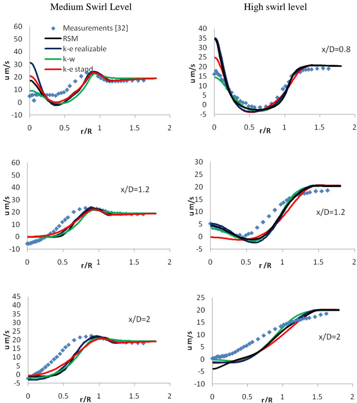
Figure 4. Radial profile of axial velocity distribution at different locations. Left column: medium swirl level (N29S054), right column: high swirl level (N16S159).
