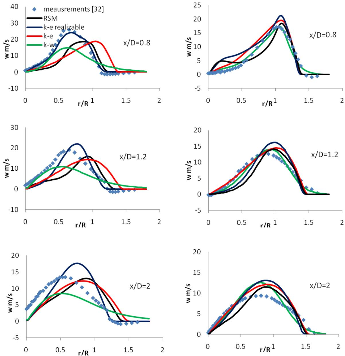
Figure 5. Radial profile of swirl velocity distribution at different locations. Left column: medium swirl level (N29S054), right column: high swirl level (N16S159).
