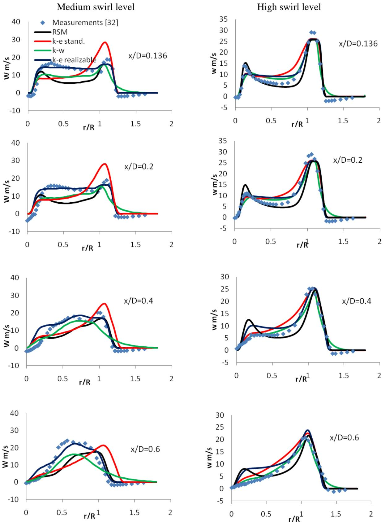
Figure 5. Radial profile of swirl velocity distribution at different locations. Left column: medium swirl level (N29S054), right column: high swirl level (N16S159).
