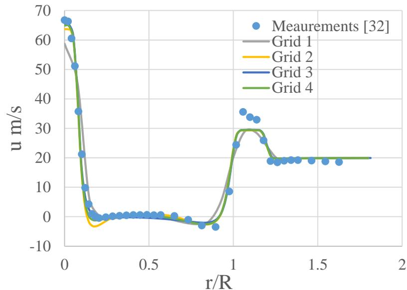
Figure 3: Radial profile of predicted axial velocity at location  $x=6.8$  mm ( $x/D=0.136$ )
