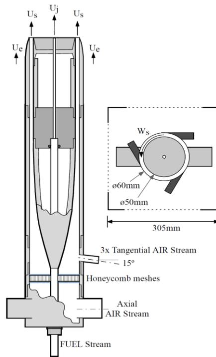
Figure1. Sydney swirl burner configuration. The figure is courtesy of [32,33]
