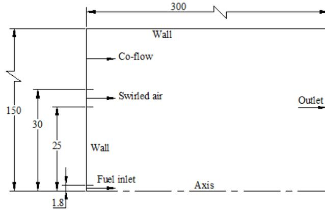
Figure 1: schematic diagram of the geometry used in the simulation. All dimensions in mm.
