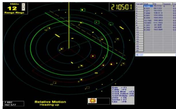
FIG. 6 RADAR DISPLAY NOT USE GYROCOMPASS INPUT
