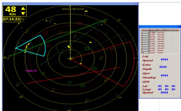
FIG. 5 RADAR DISPLAY USE GYROCOMPASS INPUT FROM USB
