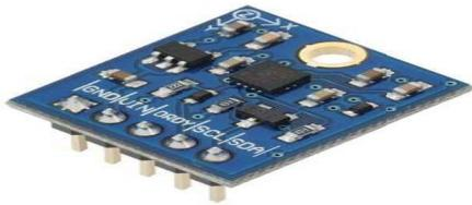
FIG.1 COMPASS MODULE WITH 3 -AXIS HMC5883L
