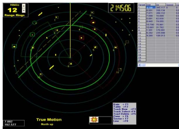
FIG. 7 RADAR DISPLAY WHEN GYROCOMPASS INPUT IMPLEMENTED
