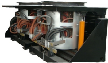
Fig. 2 Represent SEMC medium power 0.5 T induction melting furnace
