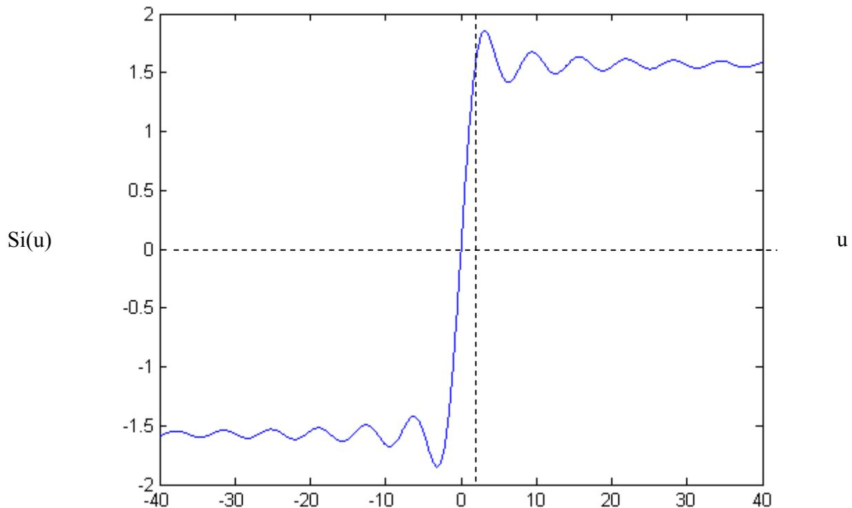
Fig.3. Sinc Integral function
