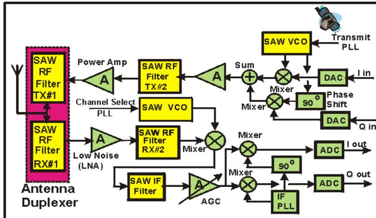
Fig.1. Basic GSM Transceiver With I-Q Modulation/Demodulation, Showing Possible SAW Components [5].
