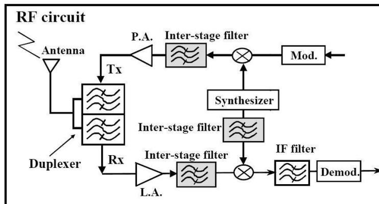
Fig.2. Duplexer Circuit with SAW components [6].
