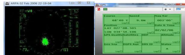
Fig. 5 Zoomed Radar Image or RADAR and GPS Image As Displayed
