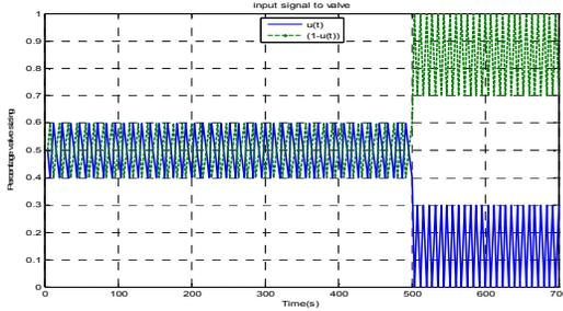
Fig. 2. Input signals for three way control valve
