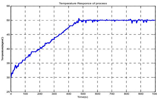
b- Adaptable PID controller response
