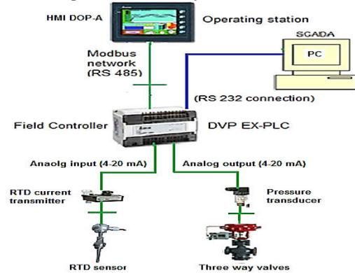
Fig. 8. The suggested automation solution
