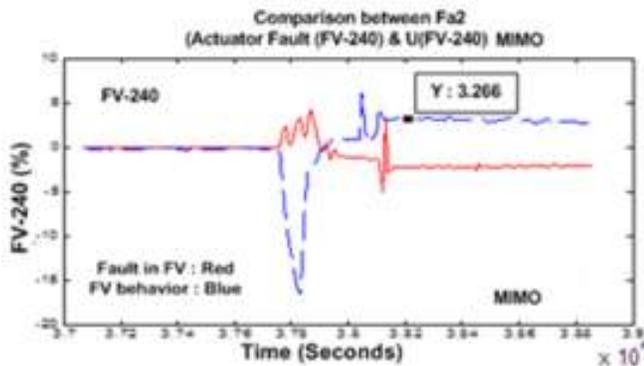
Fig. 10 real fault estimation of actuator 2
