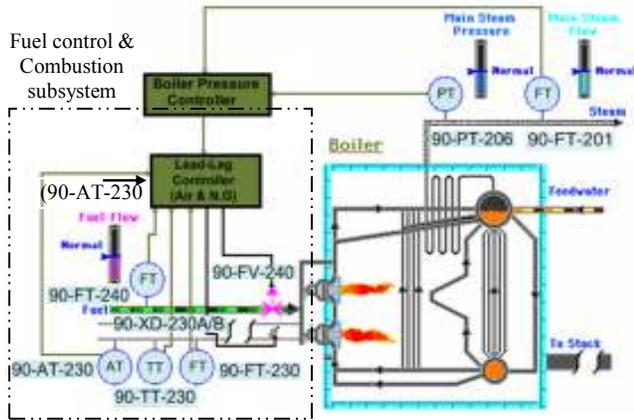
Fig. 3 Master control loop of utility boiler
