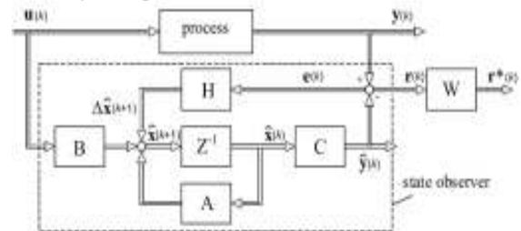
Fig. 4 Residual generation based on State observer
