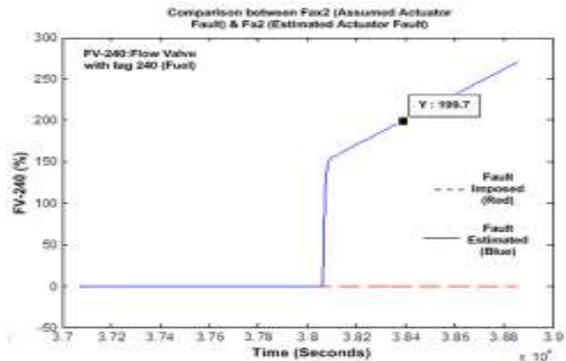
Fig. 8 Estimated fault in actuator 2 in case 1
